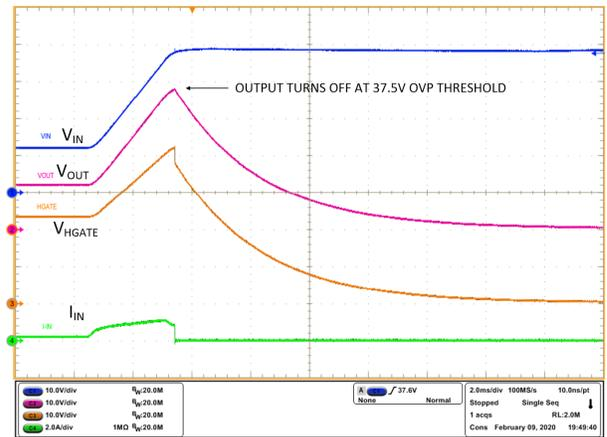
**Figure 10-18. Overvoltage Protection**
