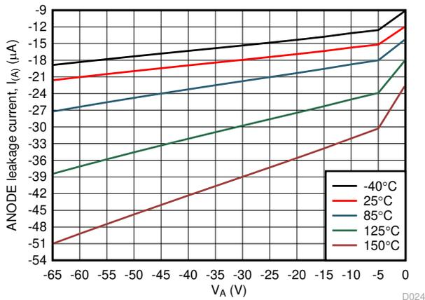
Figure 7-7. ANODE Leakage Current vs Reverse ANODE Voltage
