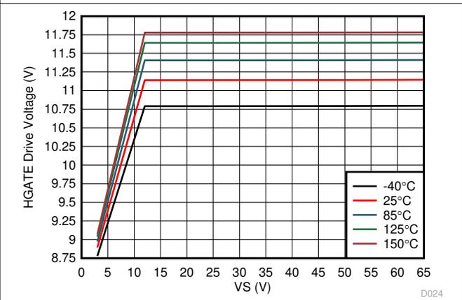
Figure 7-6. HGATE Drive Voltage vs Supply Voltage
