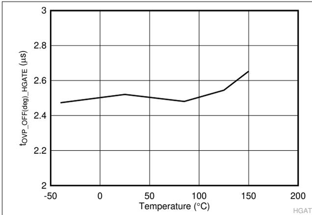
Figure 7-13. HGATE Turn OFF Delay during OV
