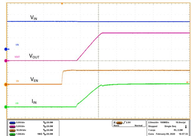
Figure 10-12. Inrush Current with 60-Ω Load
