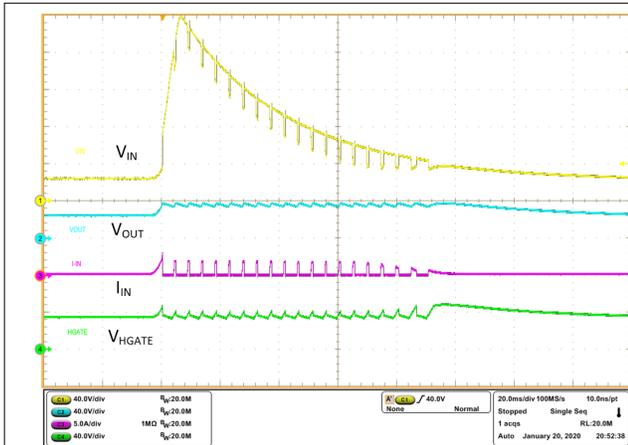
**Figure 10-26. Unsuppressed Load Dump 200 V - Output Clamp**
