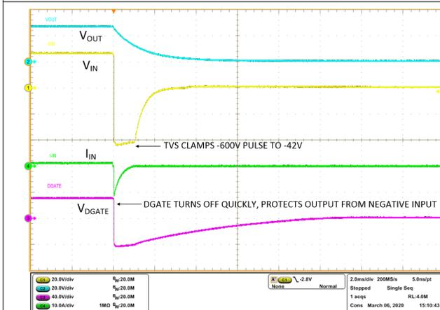
**Figure 10-28. ISO 7637-2 Pulse 1 –600 V 50 Ω**
