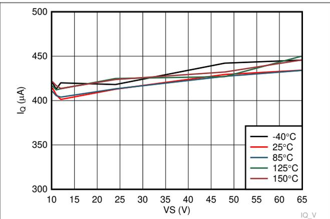
Figure 7-2. Operating Quiescent Current vs Supply Voltage (> 10 V)
