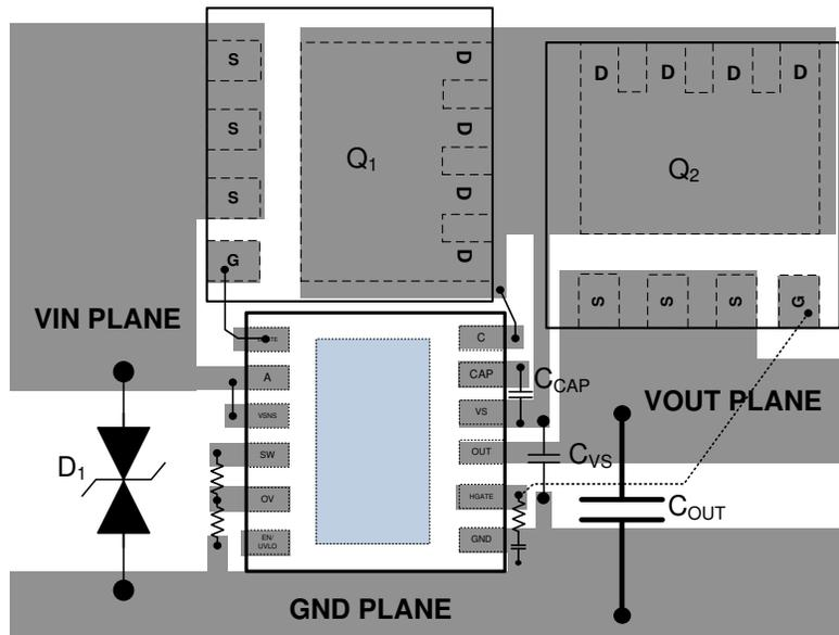
Figure 12-1. PCB Layout Example for Common Drain Configuration
