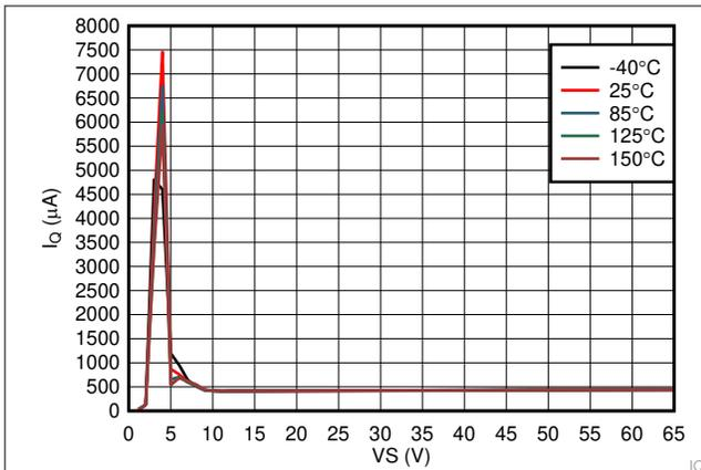
Figure 7-1. Operating Quiescent Current vs Supply Voltage
