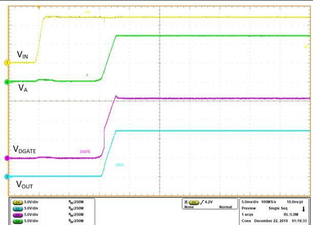
**Figure 10-31. Power up 12 V - DGATE and A**
