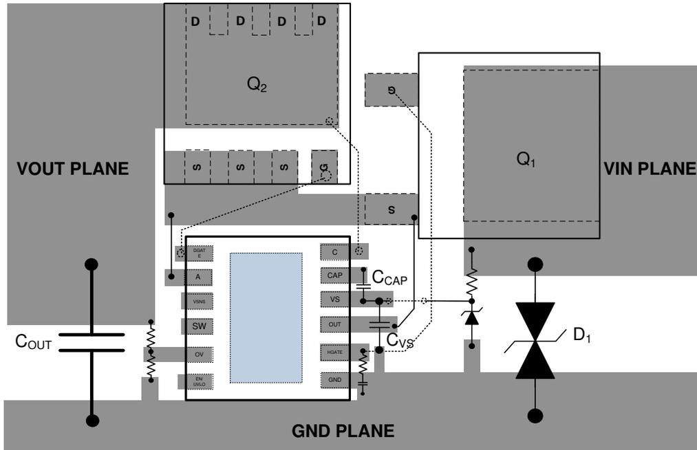
Figure 12-2. PCB Layout Example for Common Source Configuration
