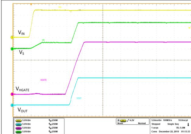
**Figure 10-30. Power up 12 V - HGATE and Output**
