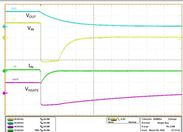
**Figure 10-29. ISO 7637-2 Pulse 1 –600 V 50 Ω**
