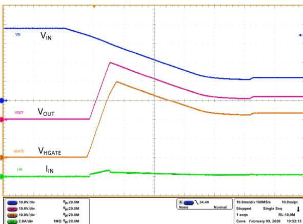
**Figure 10-19. Overvoltage Recovery**
