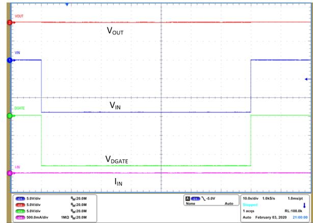
Figure 10-10. Reverse Input Voltage -14 V for 60 s
