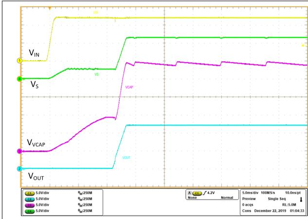
Figure 10-32. Power up 12 V - Charge Pump VCAP
