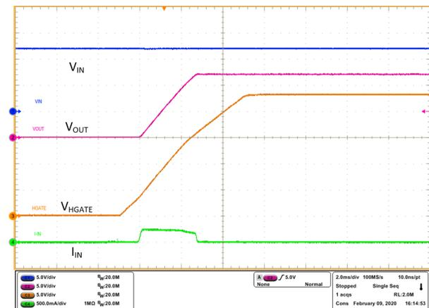
Figure 10-11. Inrush Current with no Load at Output
