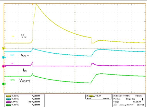
**Figure 10-27. Unsuppressed Load Dump 200 V - Output Cut-off**
