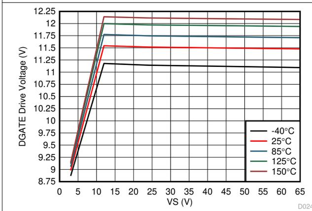
Figure 7-5. DGATE Drive Voltage vs Supply Voltage
