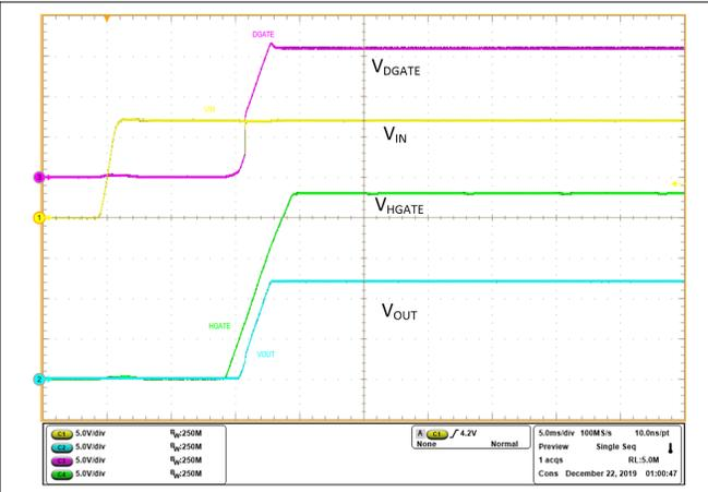
Figure 10-33. Power up 12 V - DGATE and HGATE
