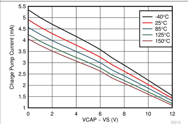
Figure 7-4. Charge Pump V-I Characteristics at VS >= 12 V
