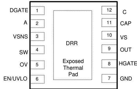
**Figure 6-1. WSON 12-Pin DRR Transparent Top View**
