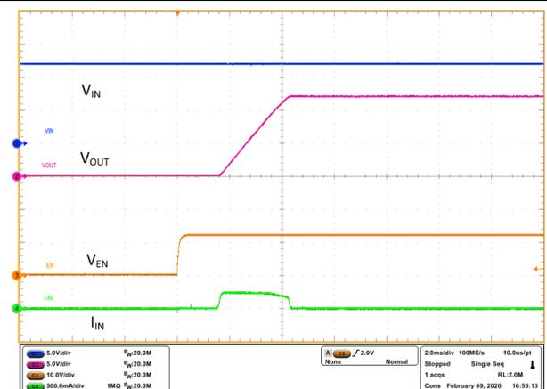
Figure 10-14. Output Turn ON with Enable
