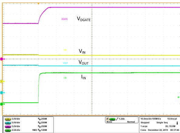
Figure 10-23. Load Transient 100 mA to 5 A
