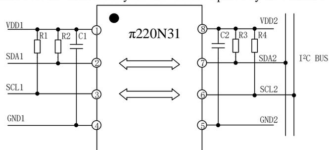
Figure 22. Typical Isolated I<sup>2</sup>C Interface Using the  $\pi$ 220N31
