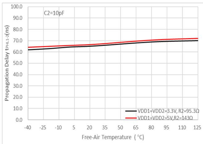
Figure 11.  $t_{PLH1-2}$  Propagation Delay vs Free-Air Temperature
