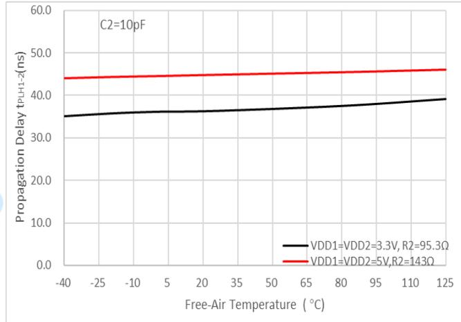
Figure 10.  $t_{PLH1-2}$  Propagation Delay vs Free-Air Temperature
