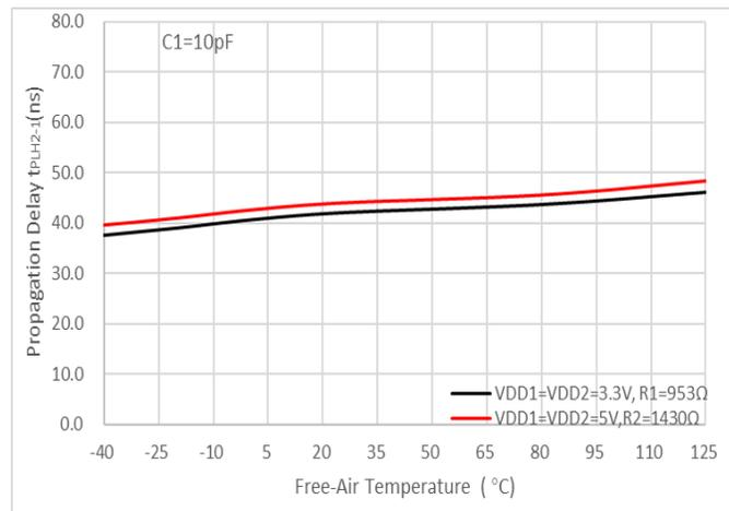
Figure 12.  $t_{PLH2-1}$  Propagation Delay vs Free-Air Temperature
