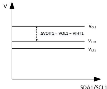
Figure 21.  $\pi$ 220N31/  $\pi$ 221N31 side 1 voltage Diagram
