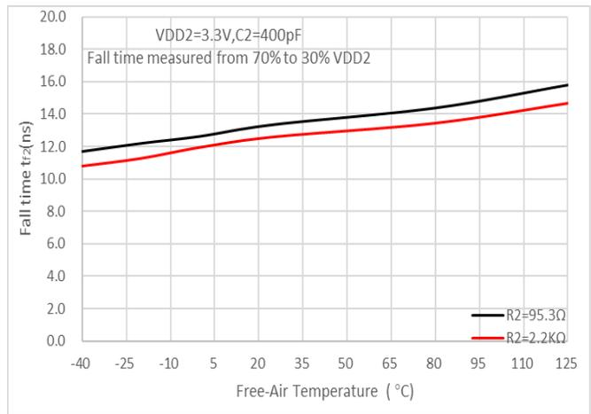
Figure 8. Side 2: Output Fall Time vs Free-Air Temperature
