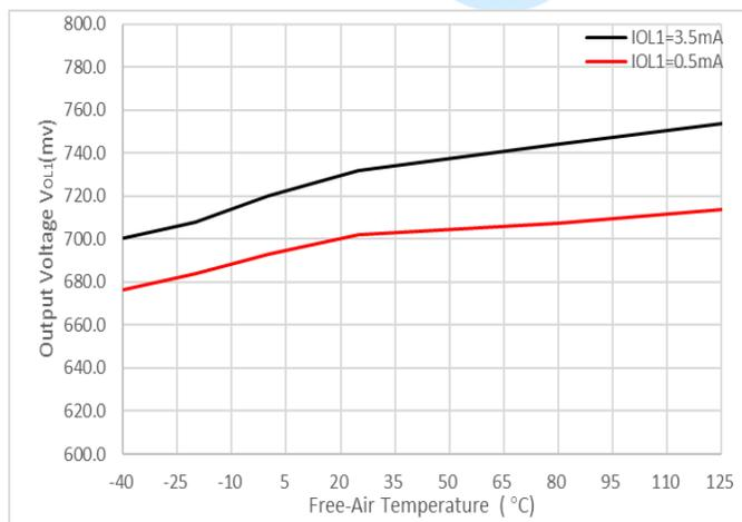
Figure 5. Side 1: Output Low Voltage vs Free-Air Temperature
