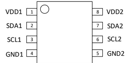
Figure 3.  $\pi$ 220N31/ $\pi$ 221N31 Pin Configuration
