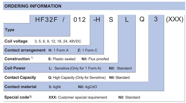
Notes: 1) Under the ambience with dangerous gas like H<sub>2</sub>S, SO<sub>2</sub> or NO<sub>2</sub>, plastic sealed type is recommended; Please test the relay in real applications. If the ambience allows, flux proofed type is preferentially recommended.
