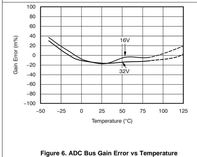
Figure 6. ADC Bus Gain Error vs Temperature
