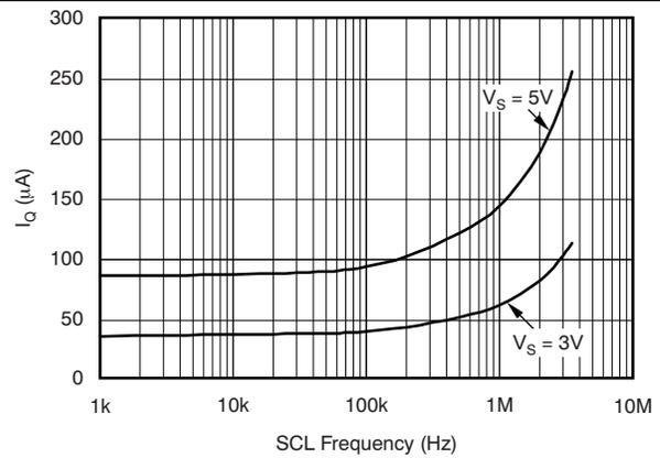
Figure 13. Shutdown  $I_Q$  vs Two-Wire Clock Frequency
