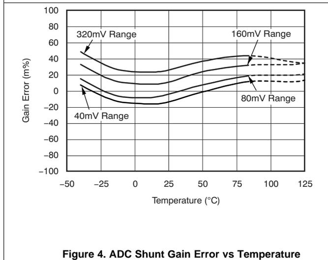
Figure 4. ADC Shunt Gain Error vs Temperature
