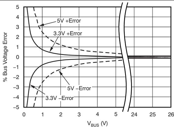
Figure 12. Total Percent Bus Voltage Error vs Supply Voltage
