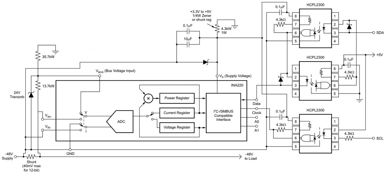
Figure 31. –48-V Telecom Current/Voltage/Power Sense With Isolation
