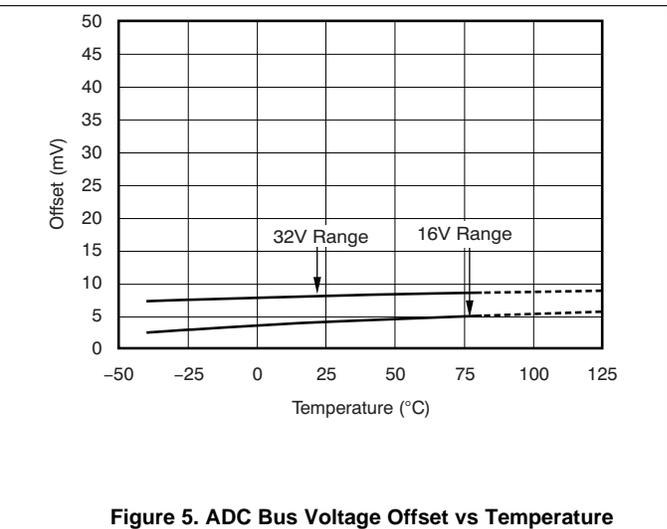
Figure 5. ADC Bus Voltage Offset vs Temperature
