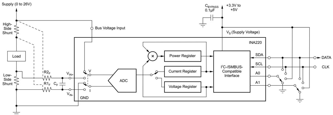
Figure 29. General Load, Low- or High-Side Sensing
