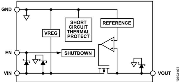
Figure 77. Fixed Output Voltage Internal Block Diagram
