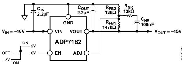
Figure 87. Noise Reduction Modification to Adjustable LDO
