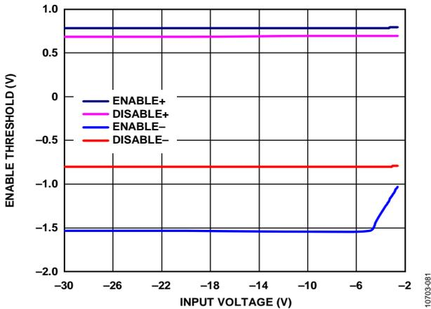
Figure 83. Typical EN Pin Thresholds vs. Input Voltage
