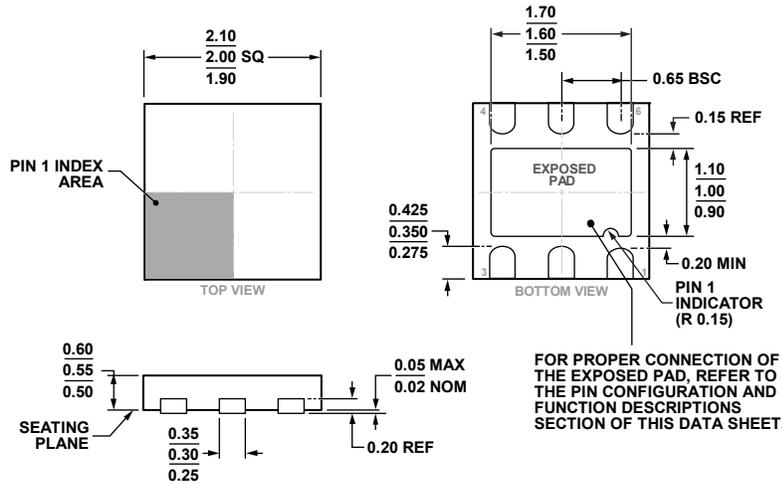
Figure 104. 6-Lead Lead Frame Chip Scale Package [LFCSPP]
