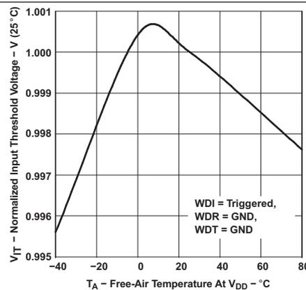
Figure 5. Normalized Input Threshold Voltage vs Free-Air Temperature at V<sub>DD</sub>
