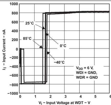
Figure 4. Input Current vs Input Voltage at WDT
