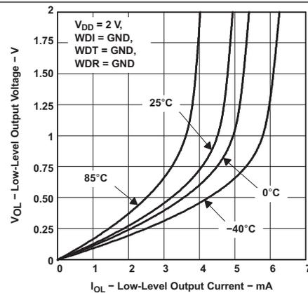
Figure 3. Low-Level Output Voltage vs Low-Level Output Current
