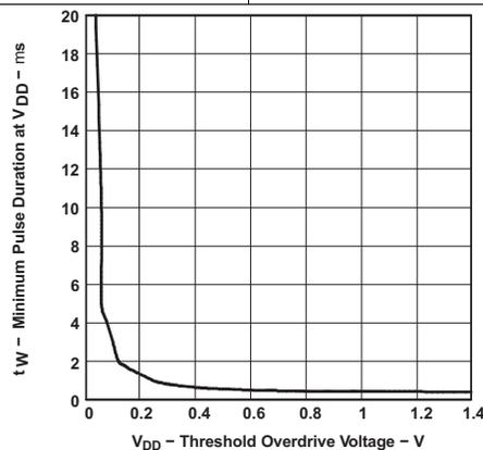
Figure 6. Minimum Pulse Duration at V<sub>DD</sub> vs V<sub>DD</sub> Threshold Overdrive Voltage
