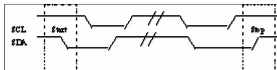
As the arrival of the start condition, master emitter must send out an address command bit, which includes slave address and R/W model; When a certain receiver in bus is chosen, it will send ACK signal and SDA changes into low voltage. ACK signal indicates the success of data transmission. When SCL clock drops, emitter sends continuously 8 bits and releases the data bus (SDA changes into high voltage).
