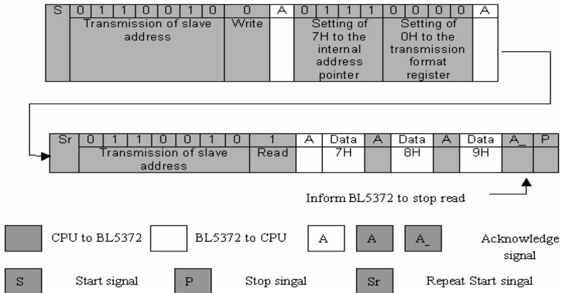
II) The second method to reading data from the internal register is to start immediately after writing to the internal address pointer and the transmission format register. Set 4h to the transmission format register when this method is used.
