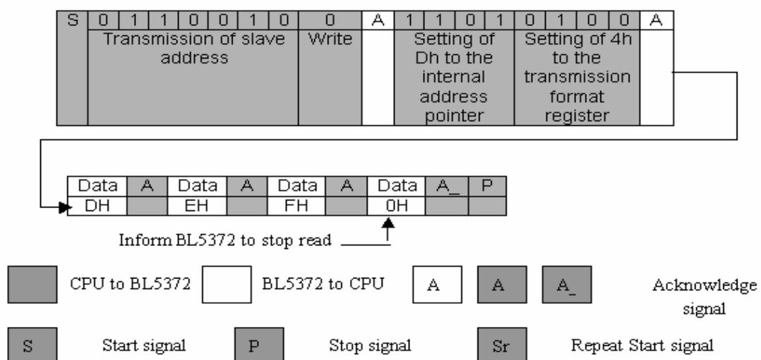
III) The third method to reading data from the internal register is to start reading immediately after writing to the slave address(0110010) and the (R/W) bit. Since the internal address pointer is set to Fh by default , this method is only effective when reading is started from the internal address Fh.
