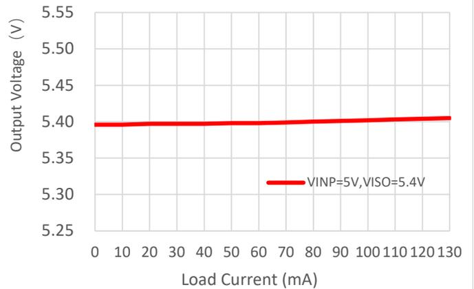
Figure 7- 18.  $V_{ISO}$  Load Regulation;  $V_{INP} = 5V$ ,  $V_{ISO} = 5.4V$
