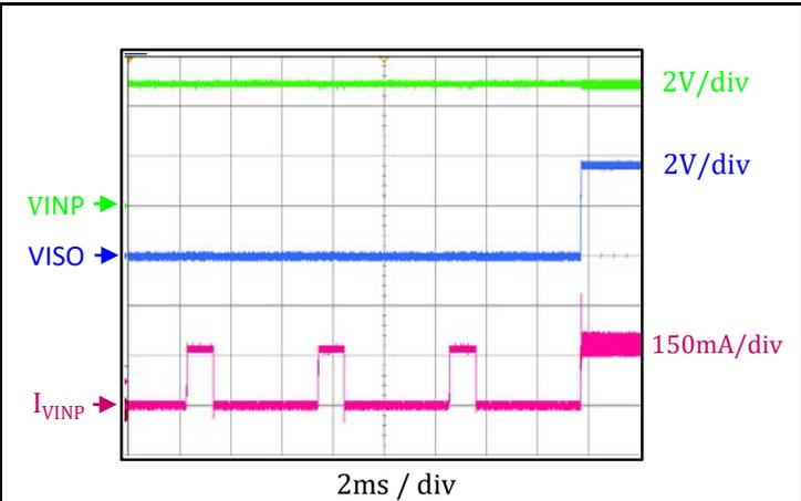
Figure 7- 8.  $V_{INP} = 5V$ ,  $V_{ISO} = 3.7V$ , output short to GNDS and recover to  $I_{ISO} = 130mA$
