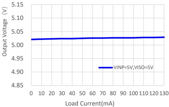
Figure 7- 17.  $V_{ISO}$  Load Regulation;  $V_{INP} = 5V$ ,  $V_{ISO} = 5V$
