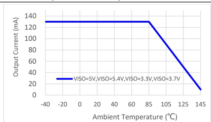
**Figure 7- 29. Maximum  $V_{ISO}$  Output Current vs. Temperature ,**
