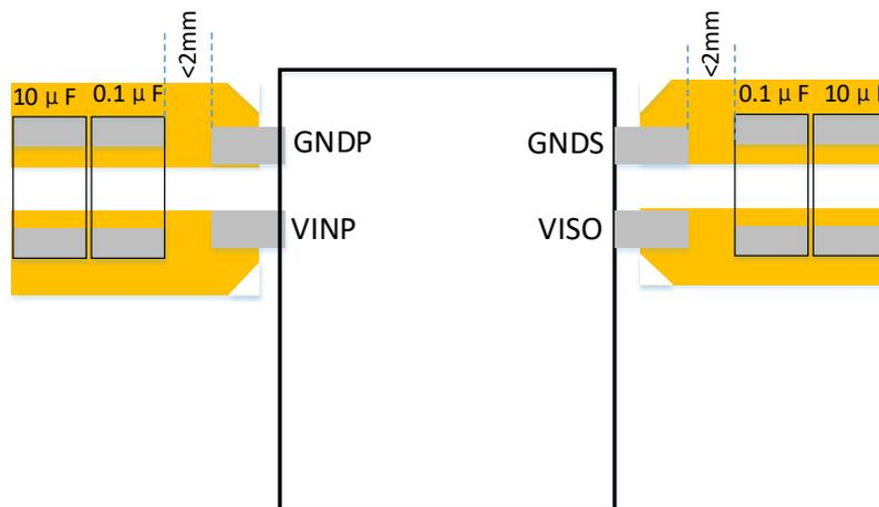
Figure 9-2. Recommended Bypass Capacitors Placement
