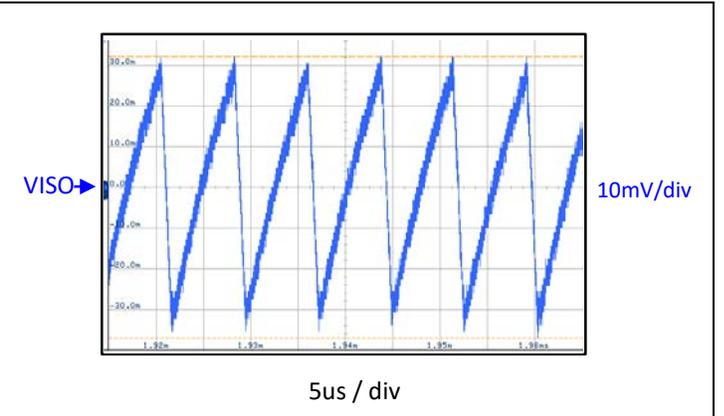
Figure7- 10  $V_{INP} = 5V$ ,  $V_{ISO} = 5.4V$ ,  $I_{ISO} = 130mA$ ;
