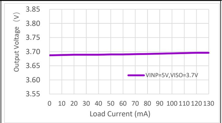
Figure 7- 20.  $V_{ISO}$  Load Regulation;  $V_{INP} = 5V, V_{ISO} = 3.7V$
