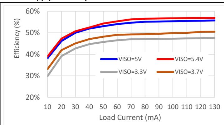
**Figure 7- 25. Power Supply Efficiency vs. Load Current**
