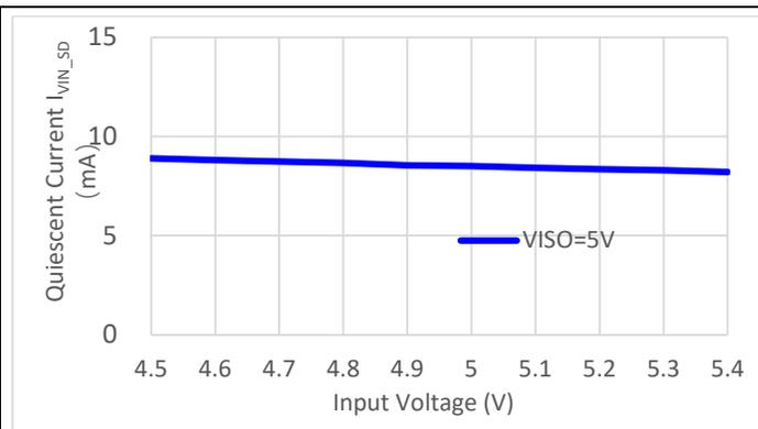
**Figure 7- 28. Quiescent Current vs. Input Voltage**
