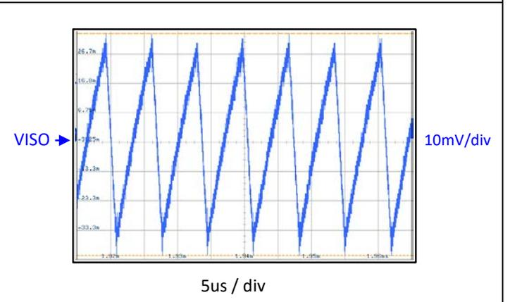
Figure 7- 12.  $V_{INP} = 5V$ ,  $V_{ISO} = 3.7V$ ,  $I_{ISO} = 130mA$ ;
