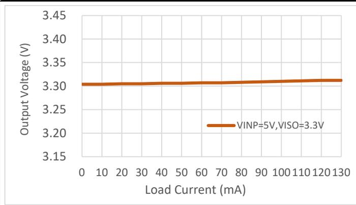
Figure 7- 19.  $V_{ISO}$  Load Regulation;  $V_{INP} = 5V, V_{ISO} = 3.3V$
