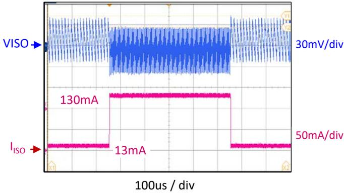
Figure 7- 13.  $V_{ISO}$  Load transient response  $V_{INP} = 5V$ ,  $V_{ISO} = 5V$ , Load step: 13mA to 130mA;  $V_{ISO}$  ripple voltage(peak to peak): 16mV
