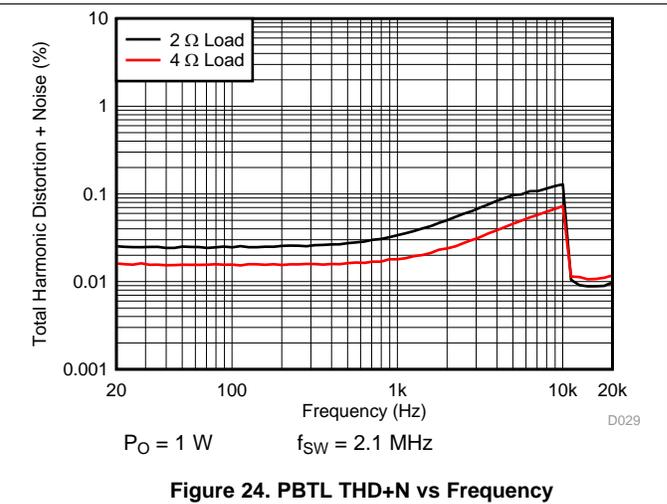
Figure 24. PBTL THD+N vs Frequency
