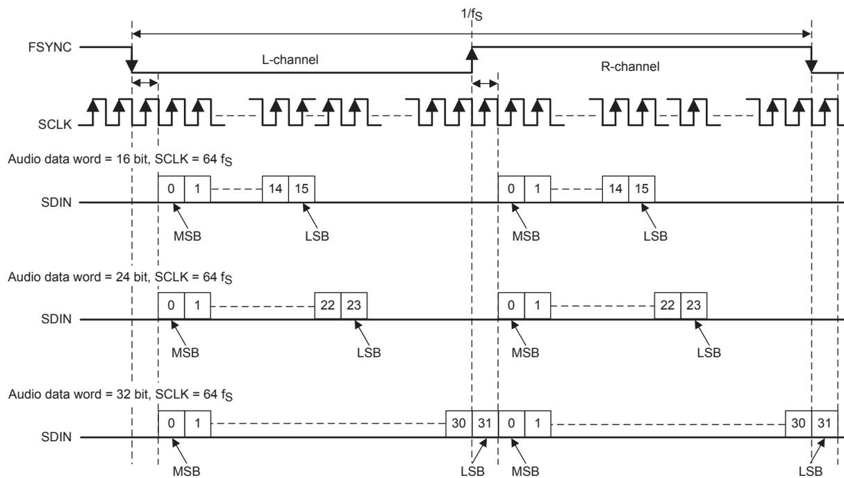
Figure 38. I<sup>2</sup>S Audio Data Format
