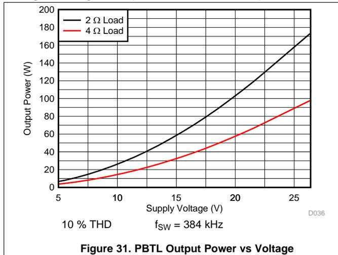
Figure 31. PBTl Output Power vs Voltage
