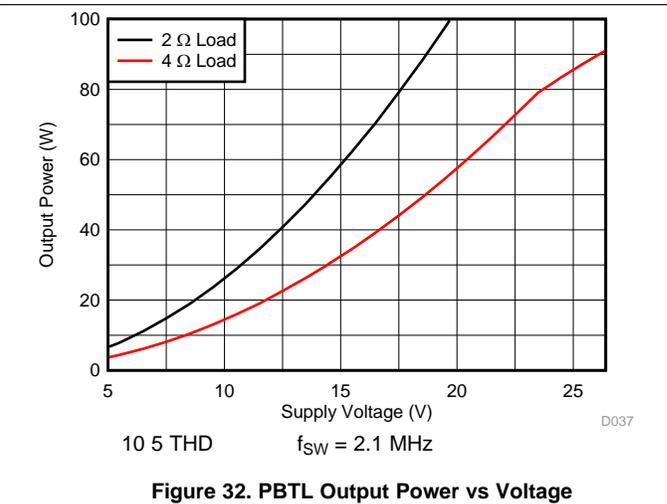
Figure 32. PBTl Output Power vs Voltage
