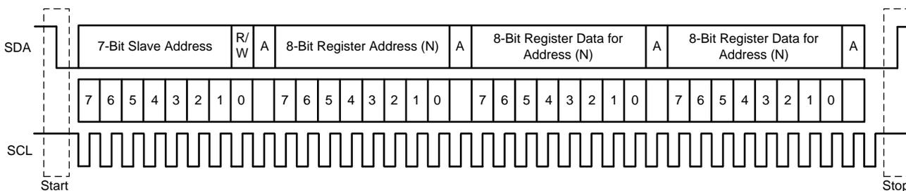
Figure 41. Typical I<sup>2</sup>C Sequence
