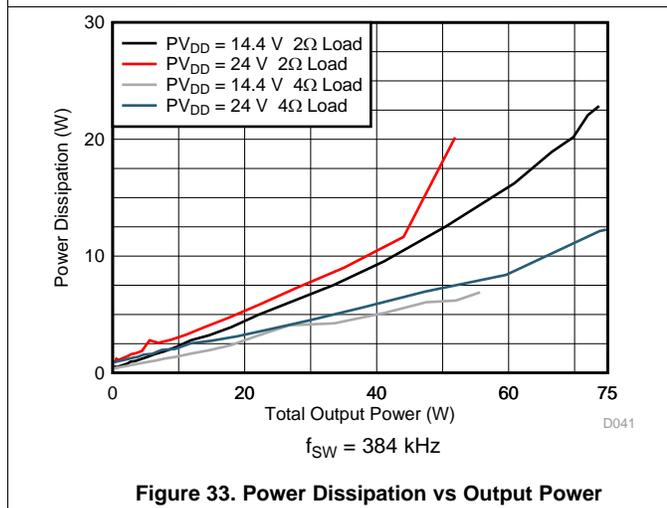
Figure 33. Power Dissipation vs Output Power
