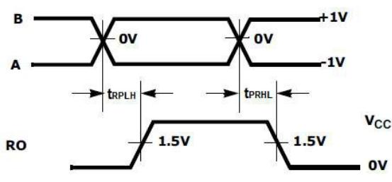
Figure 7 : Receiver Propagation Delays
