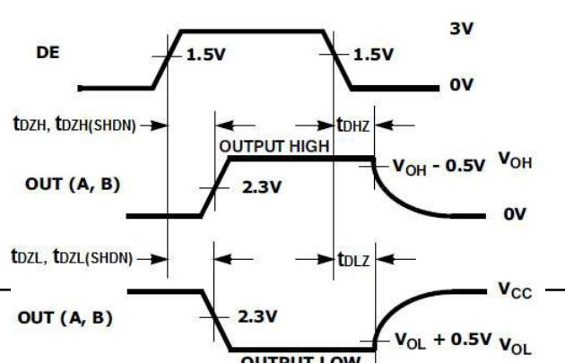
图 5: Driver Propagation Delays
