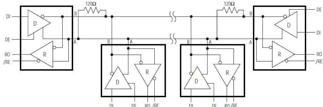
Figure 10 Typical half-duplex RS-485 network
