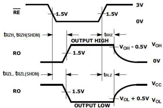
Figure 8 : Receiver Enable and Disable Times
