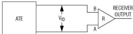
Figure 9 : Receiver Propagation Delay Test Circuit
