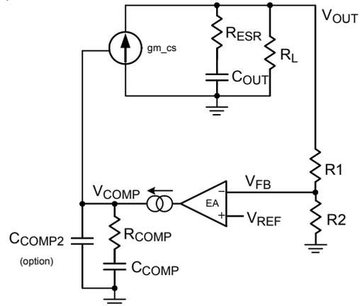
Figure 6. Simplified Equivalent Circuit of Buck with PCMC
