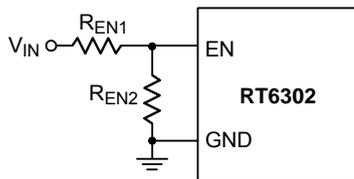
Figure 11. Resistive Divider for Under-Voltage Lockout Threshold Setting
