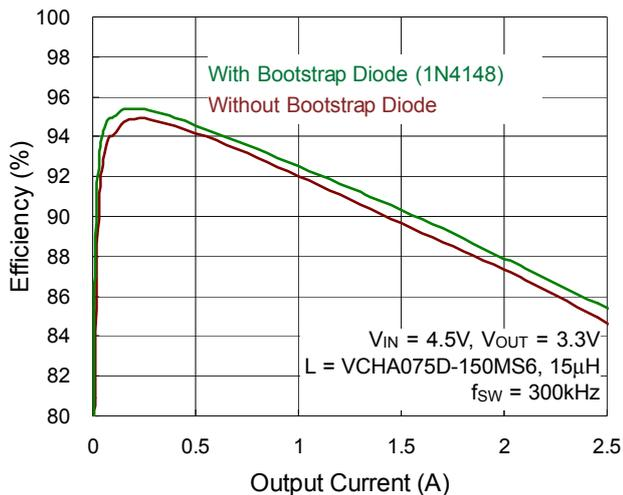
Figure 8. Efficiency Comparison between with and without Bootstrap Diode
