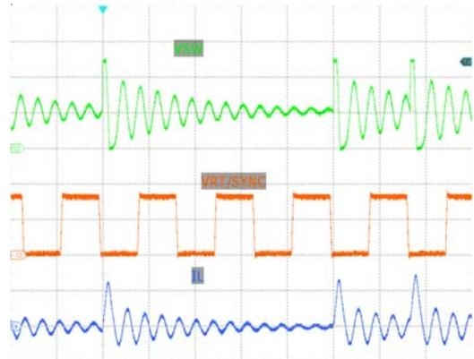
Figure 12. Synchronization Mode in PSM
