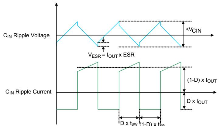
Figure 3. C<sub>IN</sub> Ripple Voltage and Ripple Current
