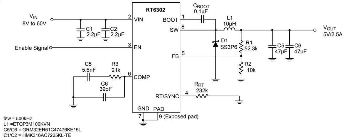
500kHz, 12V, 2.5A Step-Down Converter
