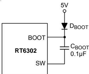
Figure 7. External Bootstrap Diode
