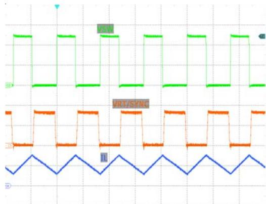
Figure 13. Synchronization Mode in CCM
