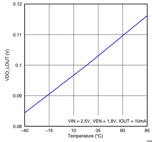
Figure 12. VDOLOUT vs Temperature VIN 2.5 V
