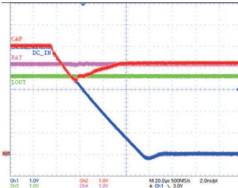
Figure 19. DC\_IN Removed, BAT Powers LDO (LOUT = 3.6 V)
