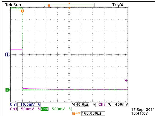
Figure 7. VOUT t<sub>OFF</sub> (No Capacitor on VOUT)
