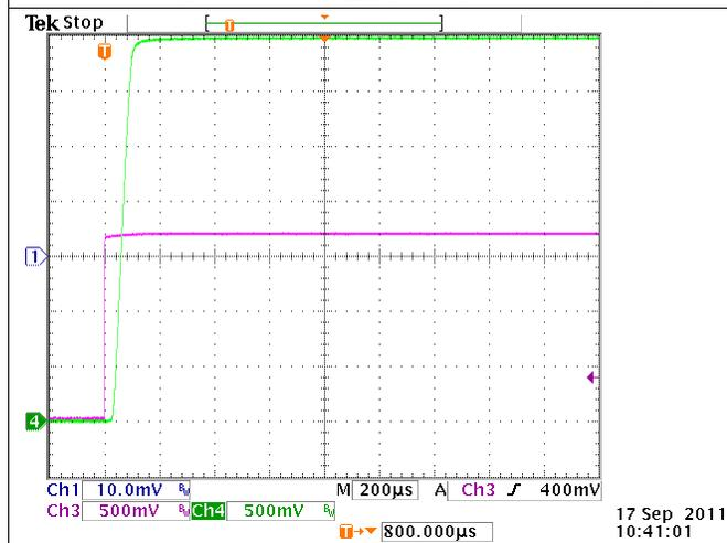
Figure 9. VOUT t<sub>ON</sub> (No Capacitor on VOUT)
