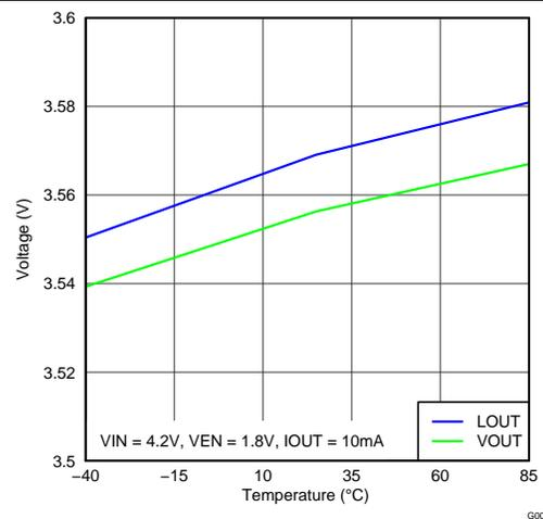
Figure 10. LOU-VOUT vs Temperature VIN 4.2 V
