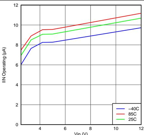
Figure 5. IIN (Operating) vs VIN
