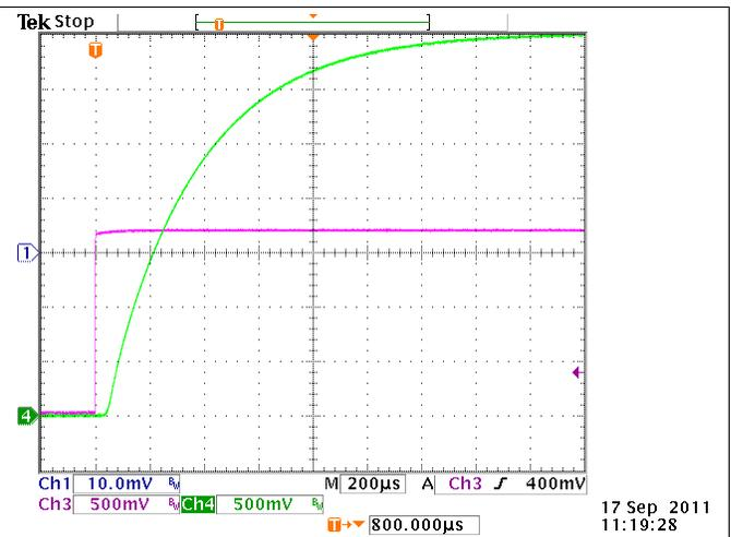
Figure 8. VOUT t<sub>ON</sub> (1 µF on VOUT)
