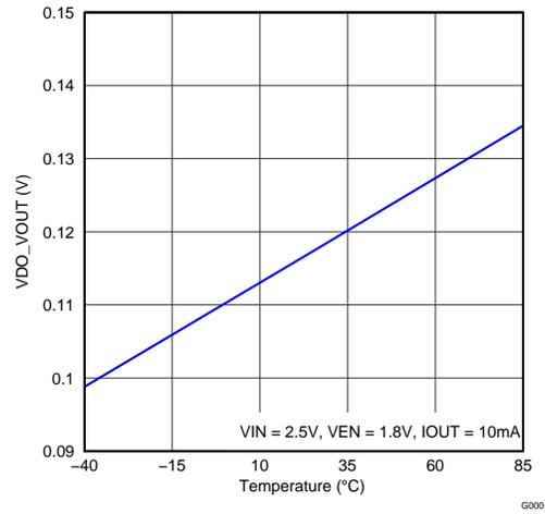
Figure 13. VDOVOUT vs Temperature VIN 2.5 V
