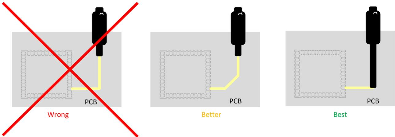
**Figure 12:** Recommended Trace Connects Antenna and the Module
