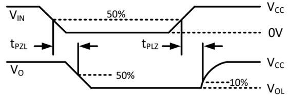
Figure 8-5. Receiver Enable and Disable Times
