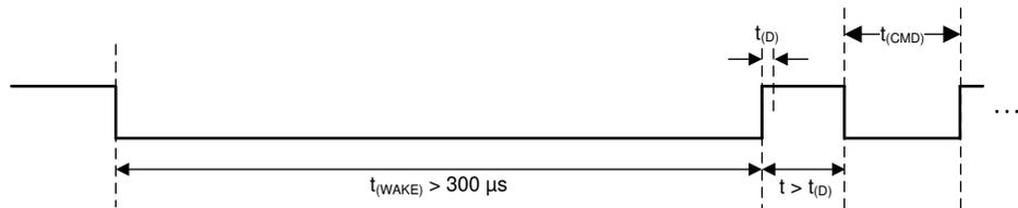
Figure 7-35. Time Command Interface Wake-Up Pulse
