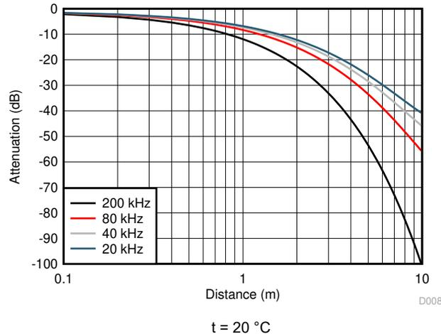
**Figure 8-2. Attenuation Characteristics of Sound Pressure by Distance**
