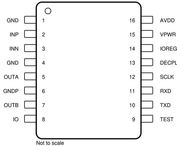
**Figure 5-1. PW Package 16-Pin TSSOP Top View**
