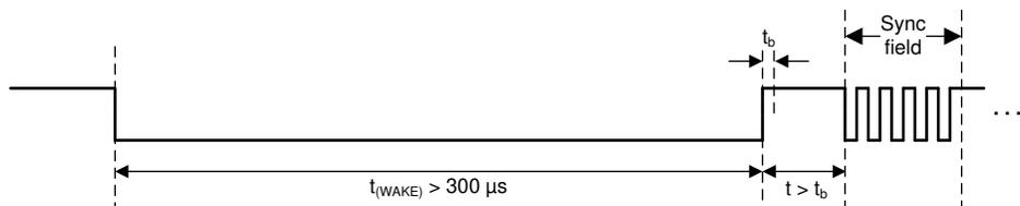
Figure 7-36. UART Wake-Up Pulse
