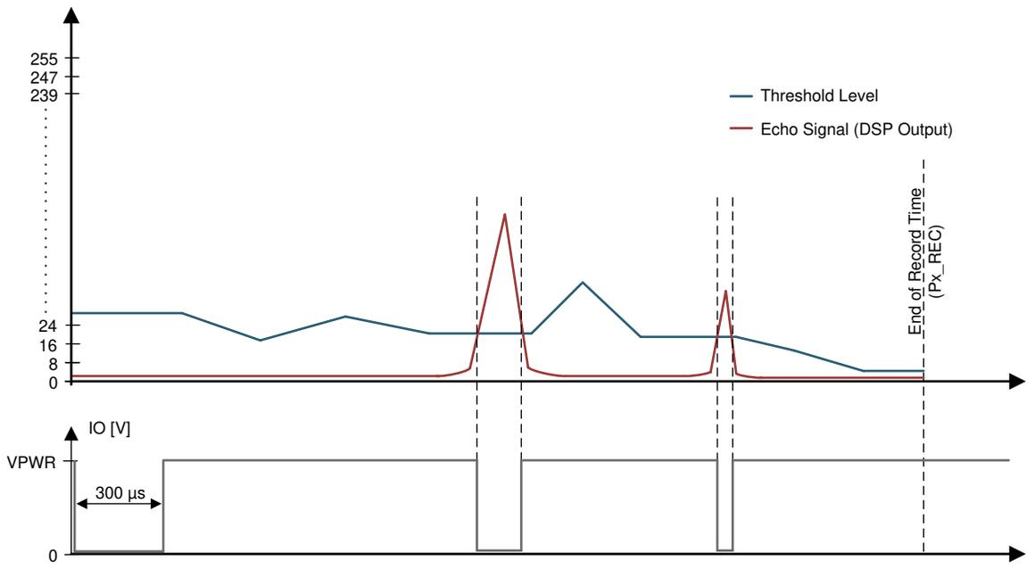
**Figure 7-14. IO-Pin Object-Detection Signaling With Listen-Only Time Command**
