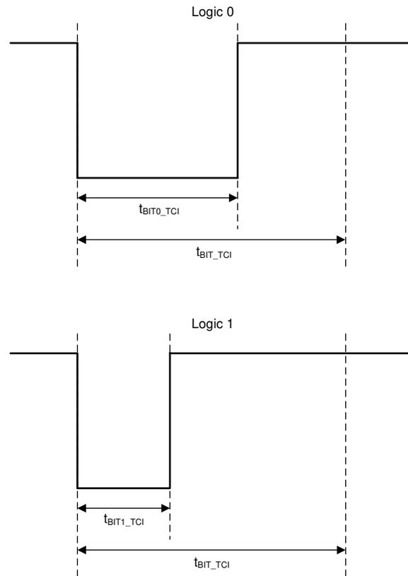
**Figure 7-11. Time-Command Interface Bit Timing**
