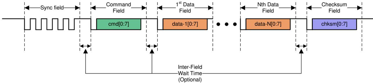
**Figure 7-20. UART Interface Transmission Frame**
