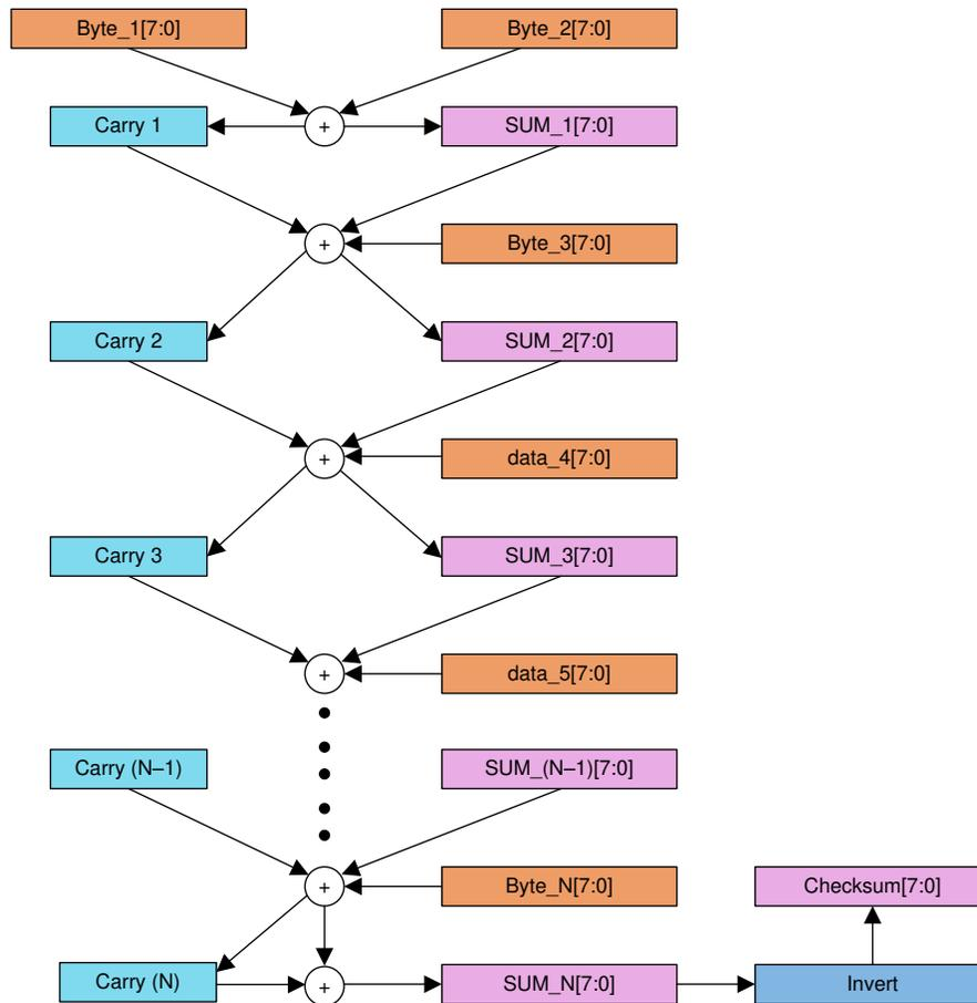
**Figure 7-17. Checksum Calculation**
