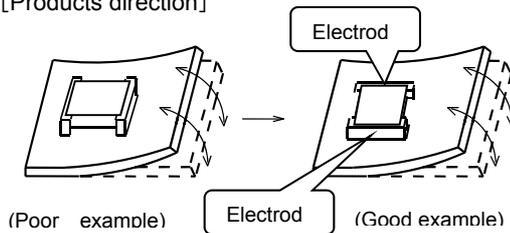
The electrode part of the products should be located like the picture to the mechanical stress.
