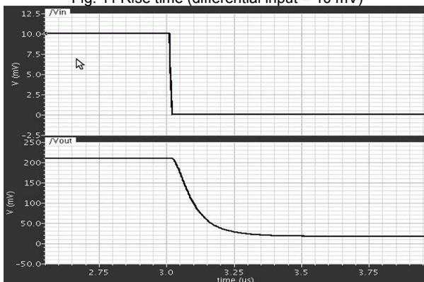
Fig. 13 Fall time (differential input = 10 mV)
