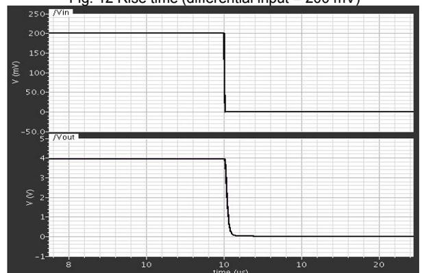
Fig. 14 Fall time (differential input = 200 mV)
