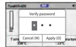
When the password switch function is enabled, entering the menu interface requires inputting the machine password. (For setting the machine password, please refer to the page 11 " Password Modification" function.)
