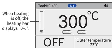
"OFF" is displayed to indicate that heating is turned off. Press the "↔" key briefly to restart heating.
