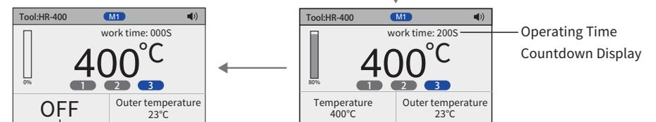
Displaying "OFF" means that the heating is turned off. Press "↔" to restart the heating.
