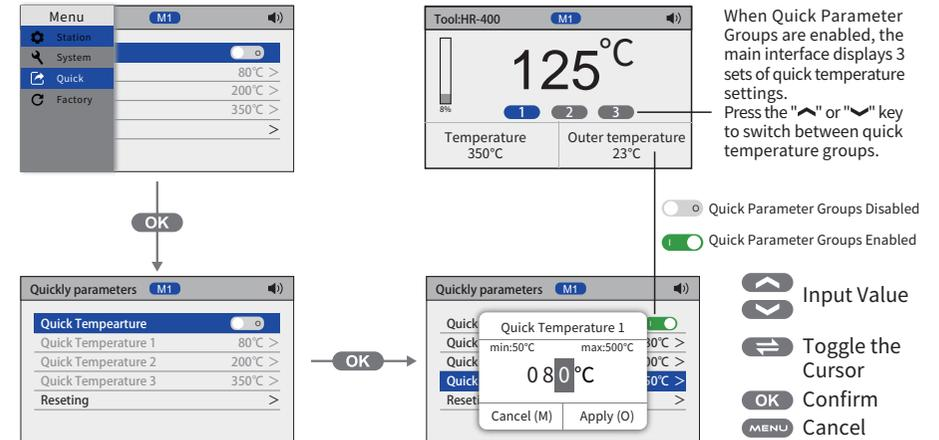
**Quick Parameter [1]:** Temperature range can be set from 50 to 500°C/122 to 932°F.
