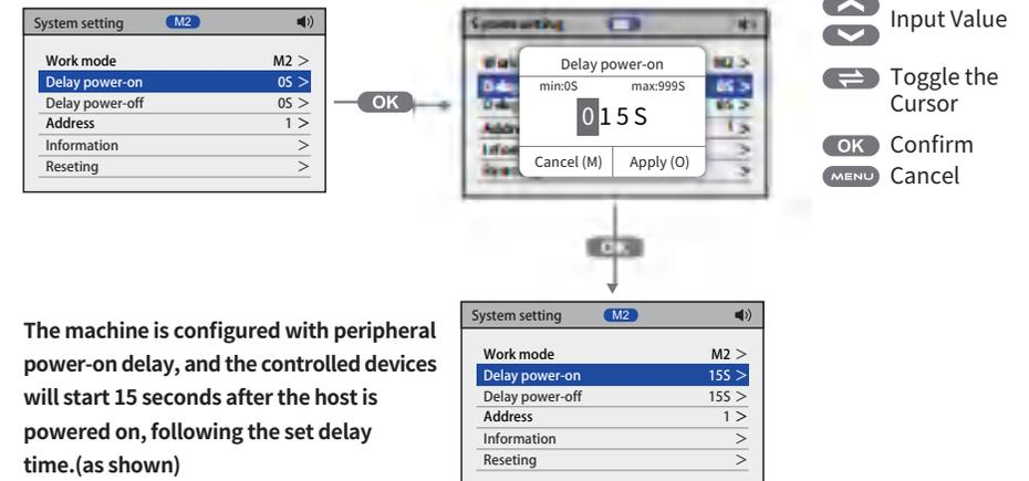
The machine is configured with peripheral power-on delay, and the controlled devices will start 15 seconds after the host is powered on, following the set delay time.(as shown)
