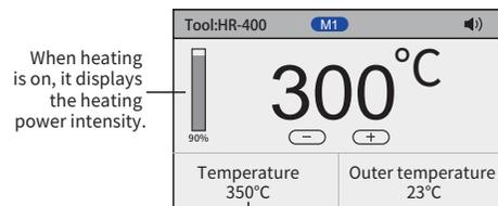
"Setting temperature value" is displayed when heating is turned on. Press the "↔" key briefly to turn off the heating.
