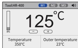
Short press "MENU" on the main interface to access the menu page. The selectable functions include preheating platform settings, system settings, quick parameters, and factory reset (as shown).
