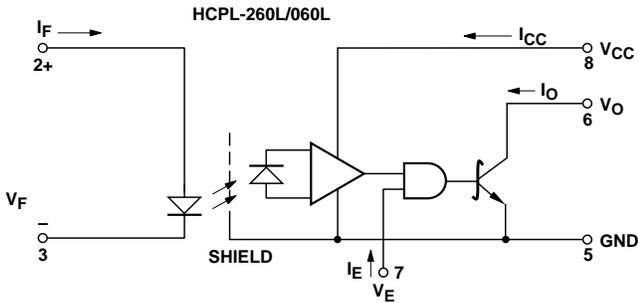
USE OF A 0.1  $\mu$ F BYPASS CAPACITOR CONNECTED BETWEEN PINS 5 AND 8 IS RECOMMENDED (SEE NOTE 5).
