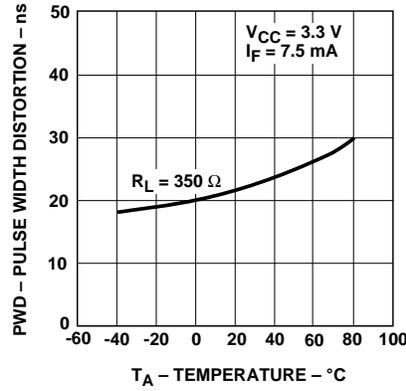
Figure 8. Typical pulse width distortion vs. temperature.
