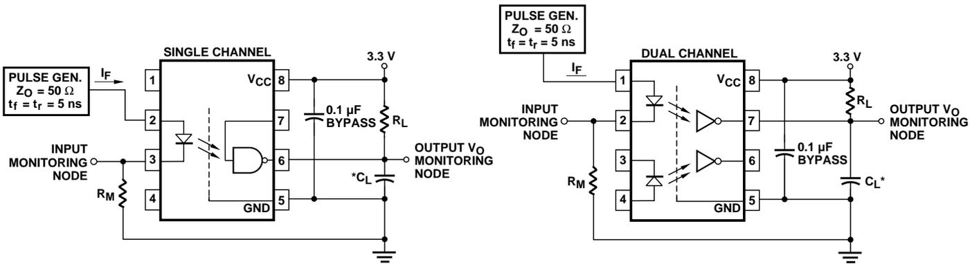
\*CL IS APPROXIMATELY 15 pF WHICH INCLUDES PROBE AND STRAY WIRING CAPACITANCE.
