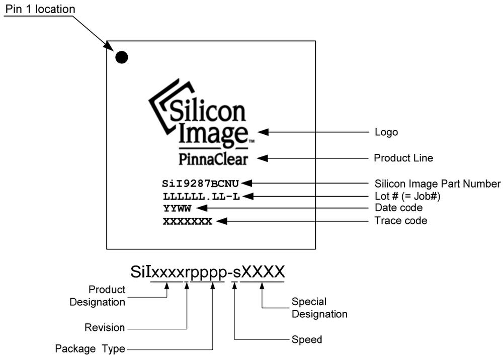
Figure 4. Marking Diagram
