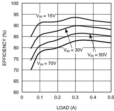
**Figure 1. LM5007 10-V Output Efficiency**
