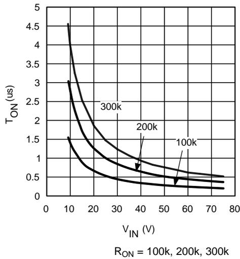
**Figure 3. VIN vs TON**
