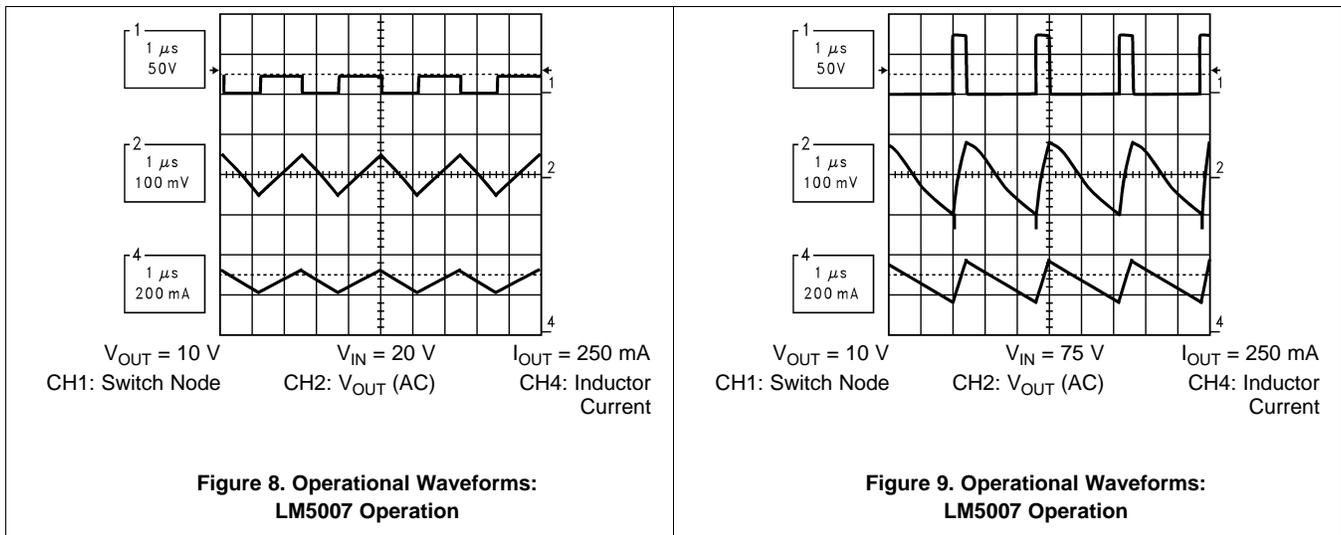
Figure 8. Operational Waveforms:
