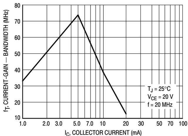
Figure 3. Current-Gain - Bandwidth
