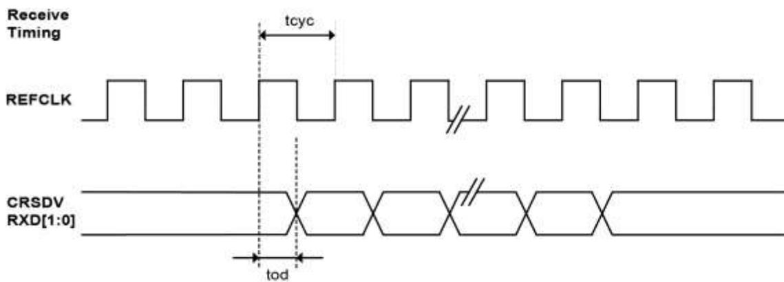
Figure 28. RMII Timing – Data Transmitted to RMII
