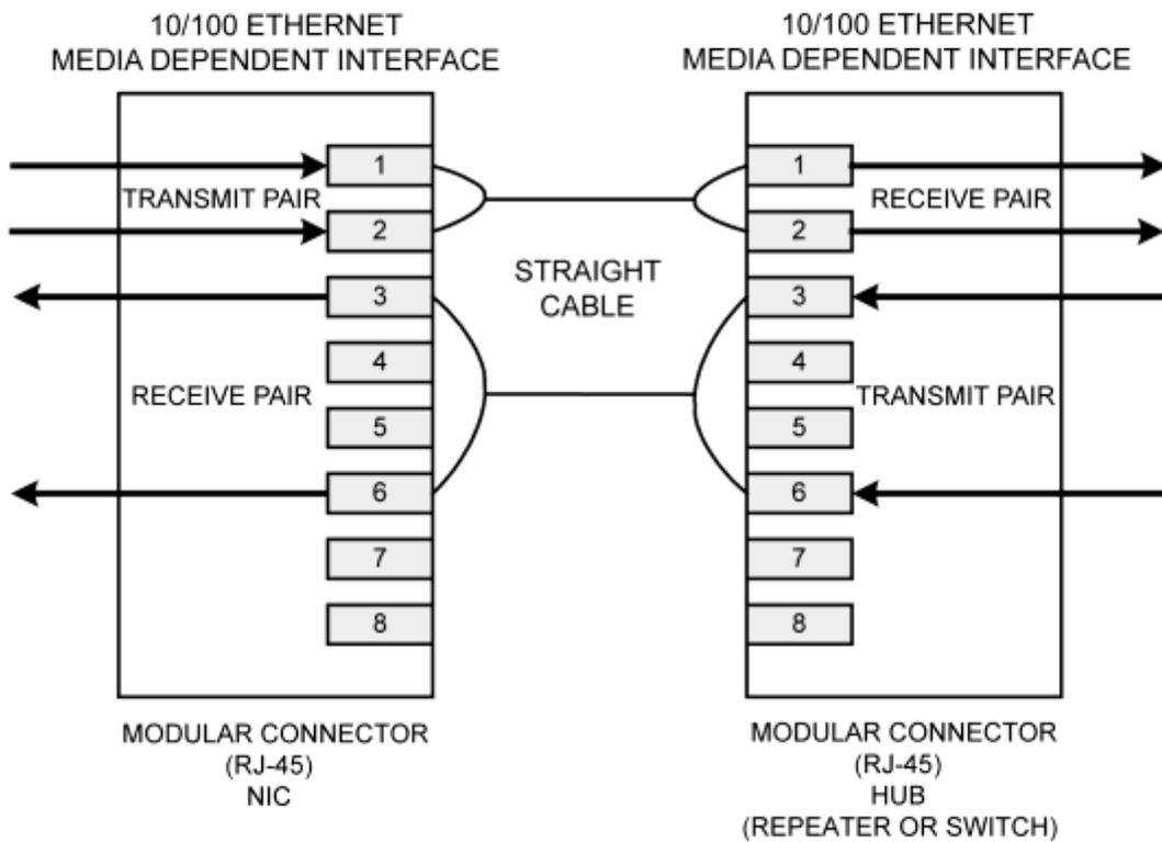
**Figure 5. Typical Straight Cable Connection**
