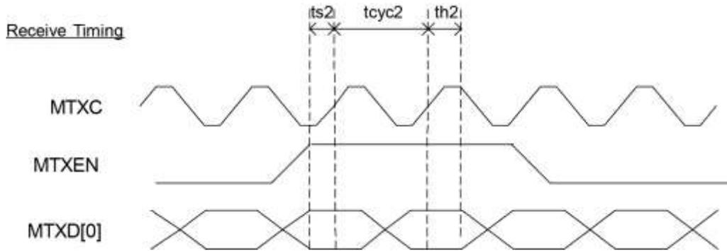
**Figure 21. SNI Input Timing**
