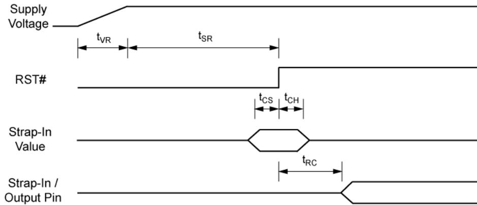
**Figure 33. Reset Timing**
