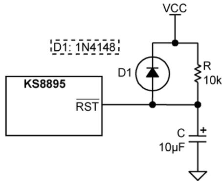
Figure 34. Recommended Reset Circuit
