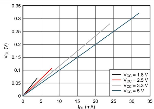
Figure 2. Typical  $V_{OL}$  vs  $I_{OL}$  -  $25^\circ\text{C}$
