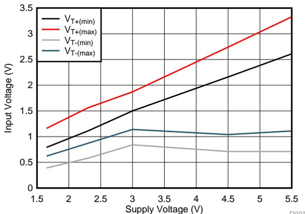
Figure 9. Interpolated Threshold Voltages vs. V<sub>CC</sub> D001
