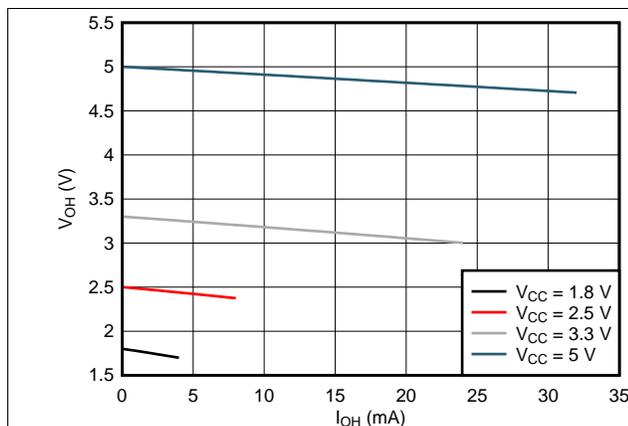
Figure 1. Typical  $V_{OH}$  vs  $I_{OH}$  -  $25^\circ\text{C}$
