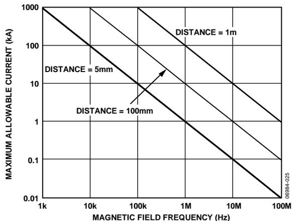
Figure 27. Maximum Allowable Current for Various Current-to-ADM2484E Spacings
