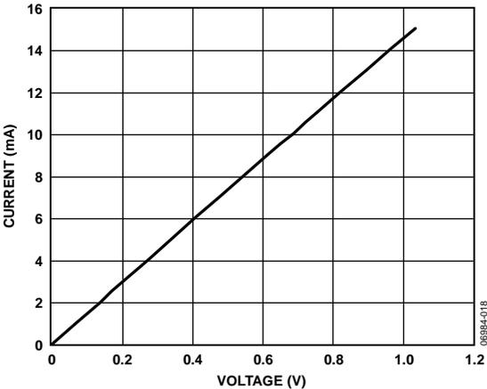
Figure 11. Output Current vs. Receiver Output Low Voltage
