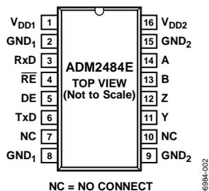
Figure 2. Pin Configuration
