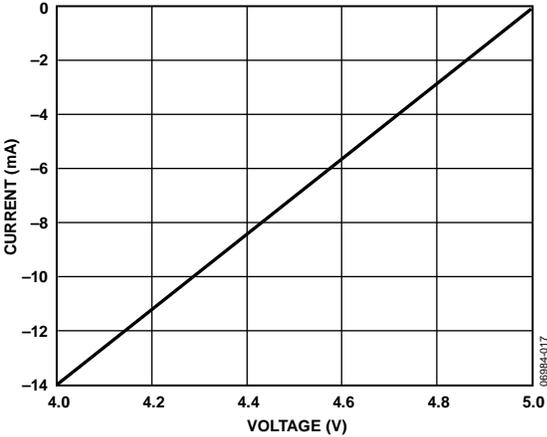
Figure 10. Output Current vs. Receiver Output High Voltage
