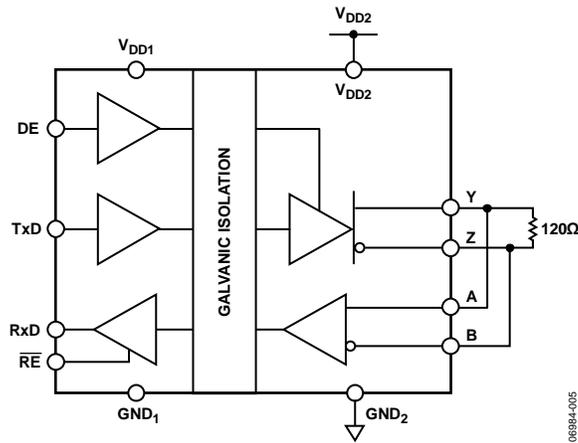
Figure 20. Supply Current Measurement Test Circuit
