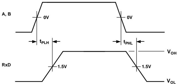
Figure 23. Receiver Propagation Delay
