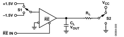
Figure 19. Receiver Enable/Disable
