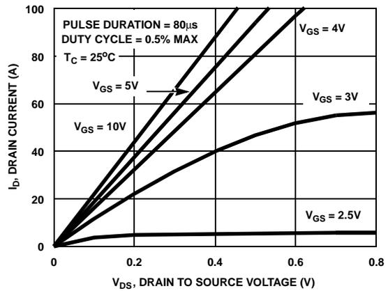
**Figure 8. Saturation Characteristics**
