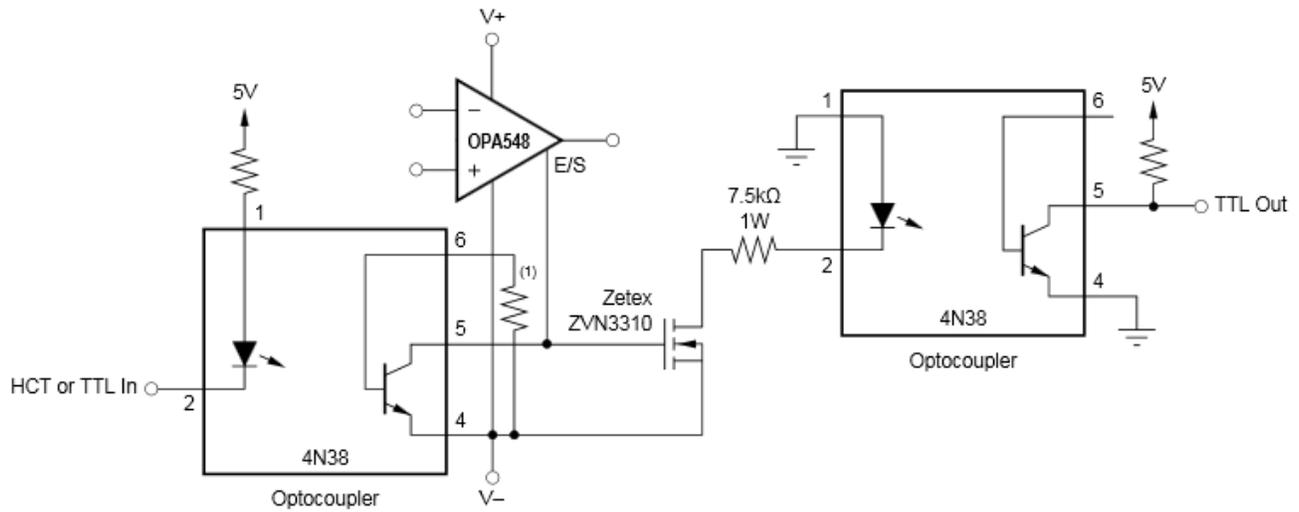
NOTE: (1) Optional—may be required to limit leakage current of optocoupler at high temperatures.
