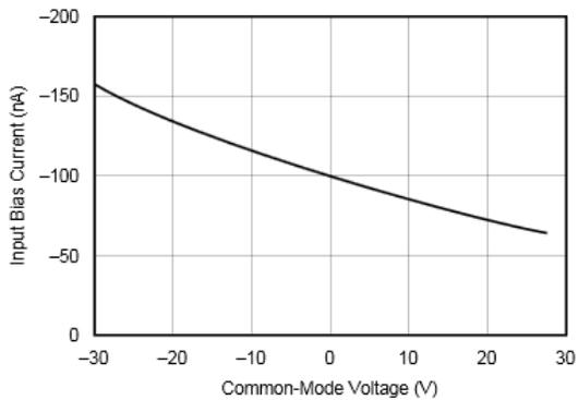
Figure 5. Input Bias Current vs Common-Mode Voltage
