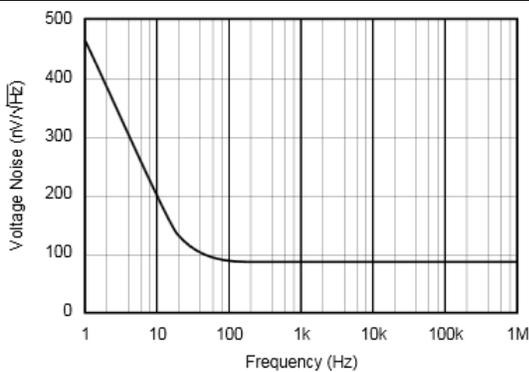
Figure 9. Voltage Noise Density vs Frequency
