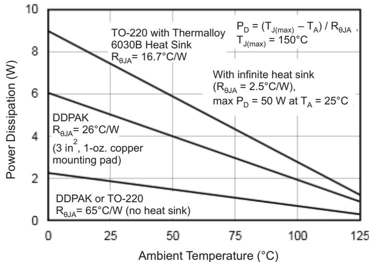
Figure 45. Maximum Power Dissipation vs Ambient Temperature
