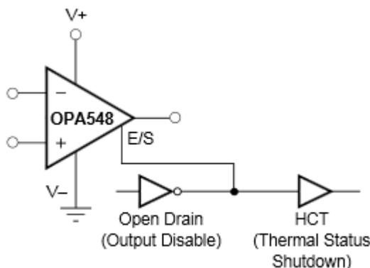
Figure 37. Output Disable and Thermal Shutdown Status With a Single Supply
