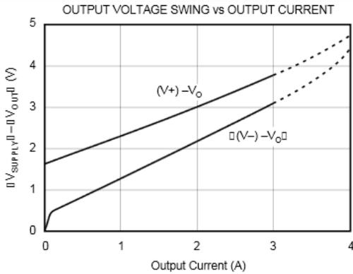
Figure 13. Output Voltage Swing vs Output Current
