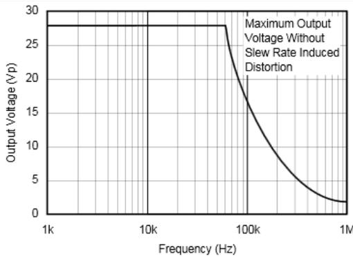
Figure 15. Maximum Output Voltage Swing vs Frequency
