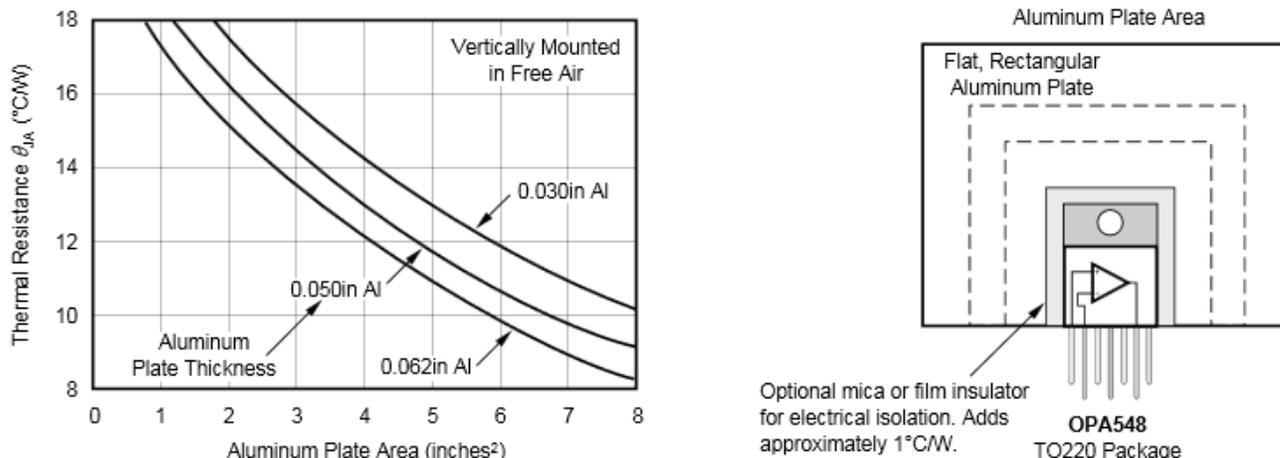
Figure 43. TO-220 Thermal Resistance vs Aluminum Plate Area
