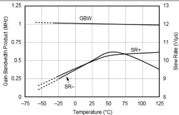
Figure 11. Gain-Bandwidth Product and Slew Rate vs Temperature
