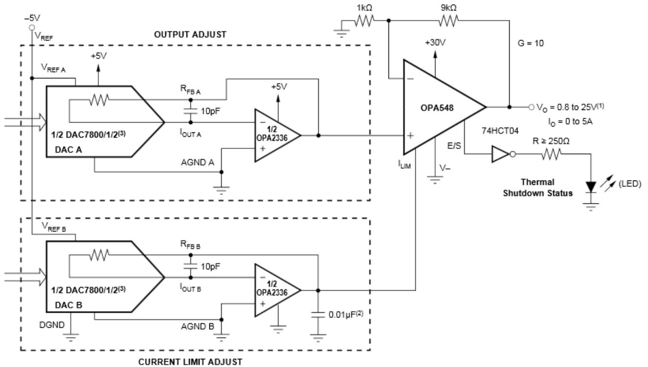
NOTES: (1) For  $V_O \leq 0V$ ,  $V_- \leq -1V$ . (2) Optional, improves noise immunity. (3) Chose DAC780X based on digital interface: DAC7800—12-bit interface, DAC7801—8-bit interface + 4 bits, DAC7802—serial interface.
