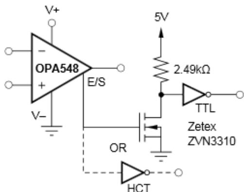
Figure 28. Thermal Shutdown Status With a Single-Supply
