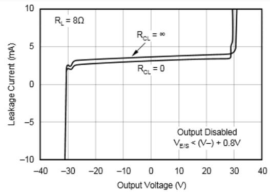
Figure 16. Output Leakage Current vs Applied Output Voltage
