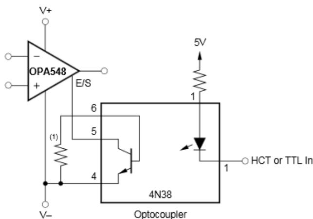
NOTE: (1) Optional—may be required to limit leakage current of optocoupler at high temperatures.
