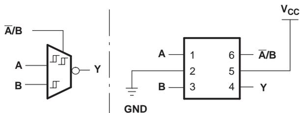
Figure 1. 2-to-1 Data Selector With Inverted Output
