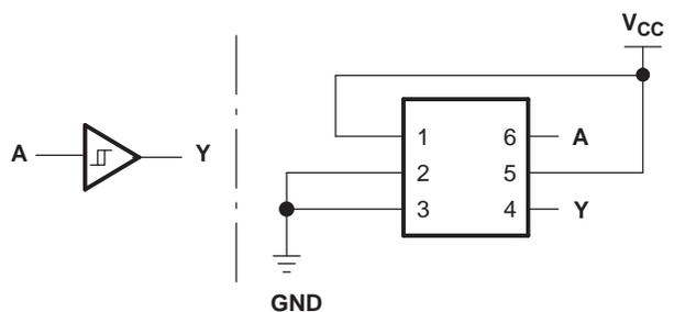
Figure 6. Noninverted Buffer
