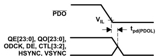
Figure 9. Delay From  $\overline{PDO}$  Low to Hi-Z Outputs
