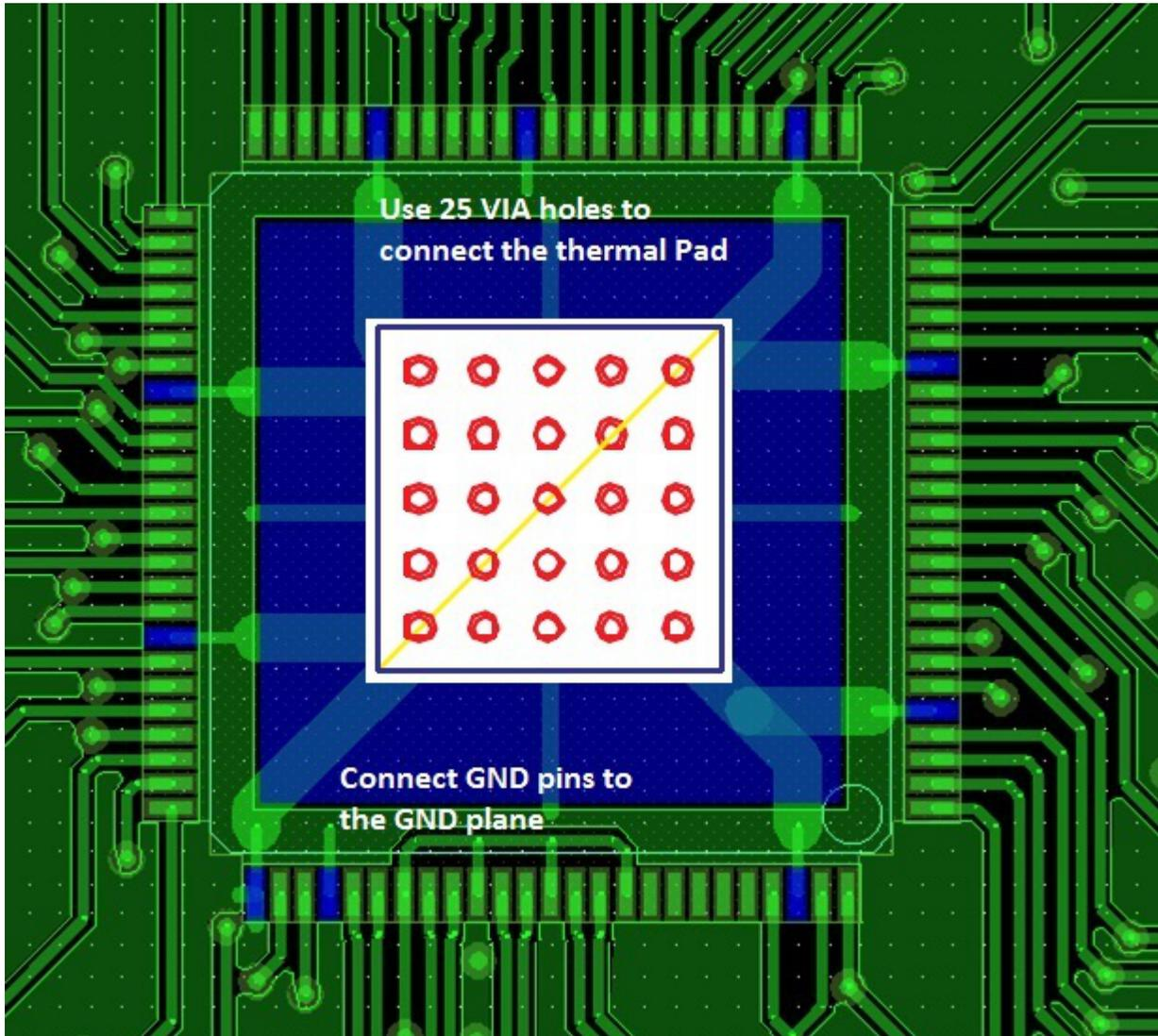
**Figure 27. Ground Routing**
