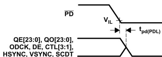
Figure 8. Delay From  $\overline{PD}$  Low to Hi-Z Outputs
