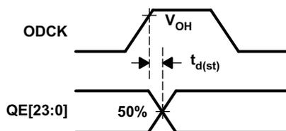
Figure 6. ODCK High to QE[23:0] Staggered Data Output
