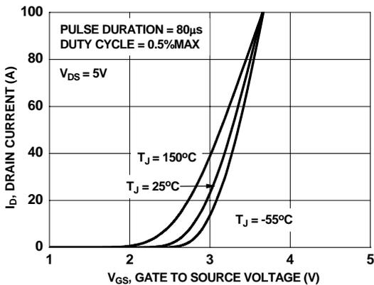
**Figure 5. Transfer Characteristics**
