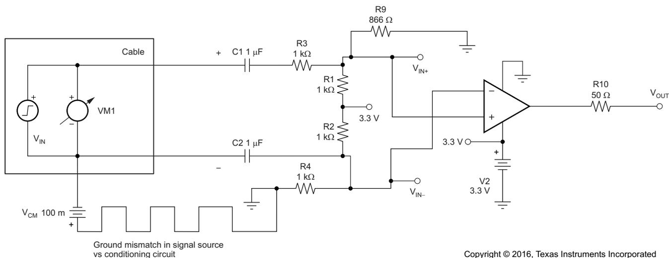
**Figure 18. TLV3491 Configured as an AC-Coupled Comparator (Schematic)**
