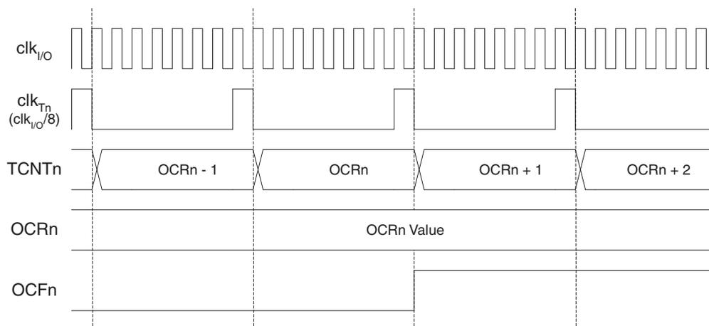
**Figure 17-11** shows the setting of OCF2 and the clearing of TCNT2 in CTC mode.
