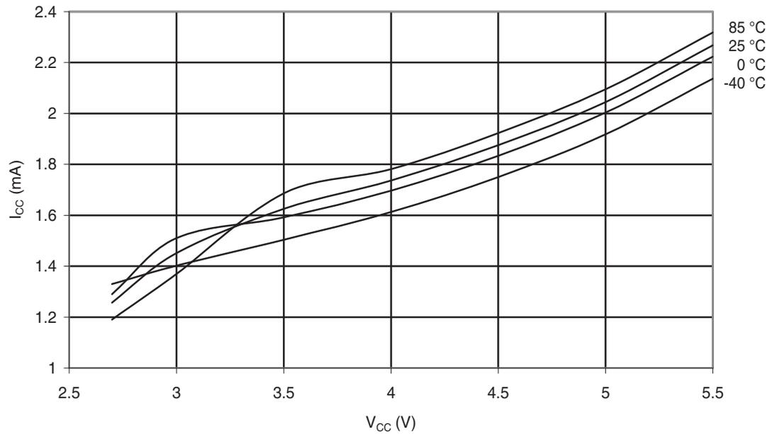
**Figure 29-4.** Active Supply Current vs.  $V_{CC}$  (Internal RC Oscillator, 2 MHz)
