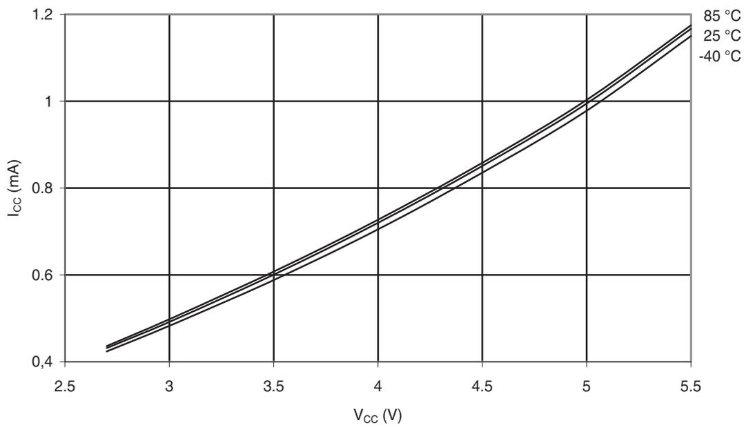
**Figure 29-12.** Idle Supply Current vs.  $V_{CC}$  (Internal RC Oscillator, 4 MHz)
