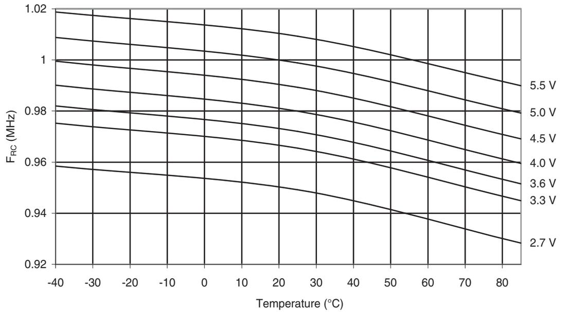
**Figure 29-41.** Calibrated 1 MHz RC Oscillator Frequency vs.  $V_{CC}$
