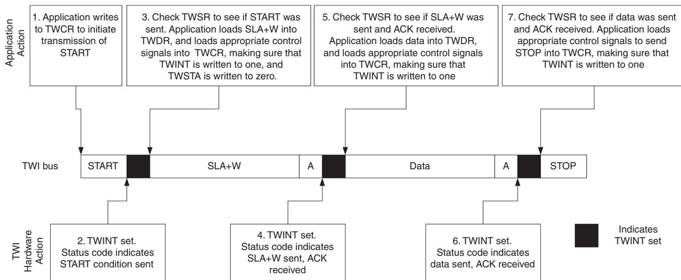
1. The first step in a TWI transmission is to transmit a START condition. This is done by writing a specific value into TWCR, instructing the TWI hardware to transmit a START condition. Which value to write is described later on. However, it is important that the TWINT bit is set in the value written. Writing a one to TWINT clears the flag. The TWI will
