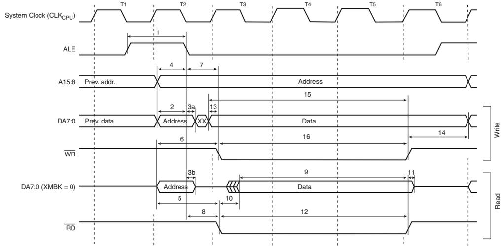
**Figure 28-9. External Memory Timing (SRWn1 = 1, SRWn0 = 1)<sup>(1)</sup>**
