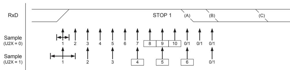
The same majority voting is done to the stop bit as done for the other bits in the frame. If the stop bit is registered to have a logic 0 value, the Frame Error n (FEn) flag will be set.
