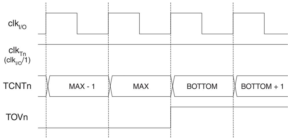
Figure 17-9 shows the same timing data, but with the prescaler enabled.
