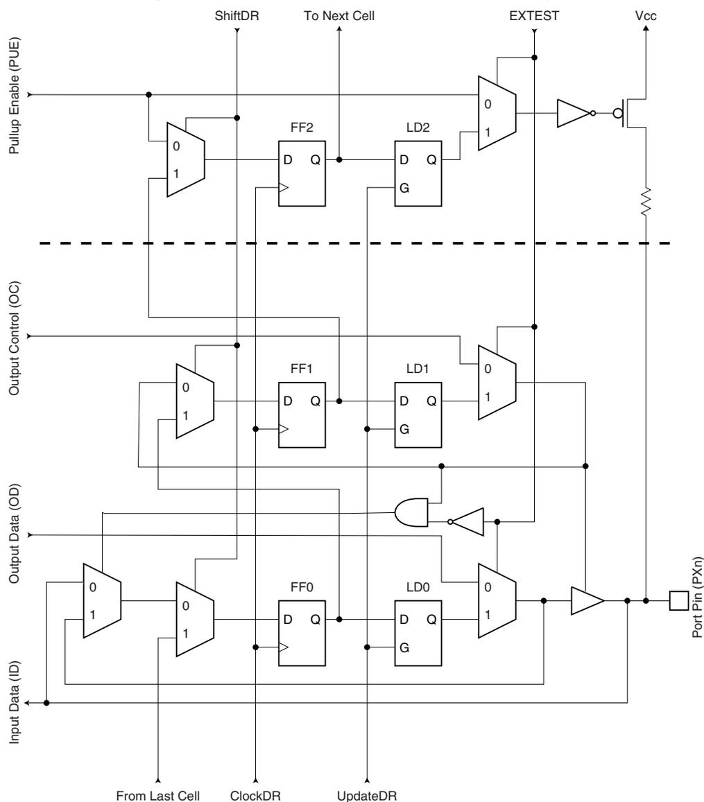
**Figure 25-4. General Port Pin Schematic Diagram**
