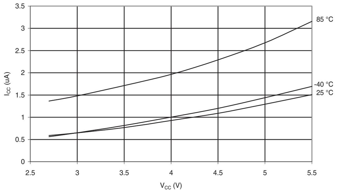
**Figure 29-16.** Power-Down Supply Current vs.  $V_{CC}$  (Watchdog Timer Enabled)
