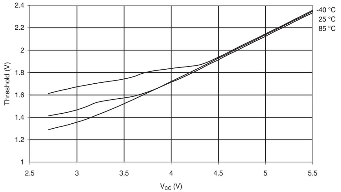
**Figure 29-34.** Reset Input Threshold Voltage vs.  $V_{CC}$  ( $V_{IL}$ , Reset Pin Read as '0')
