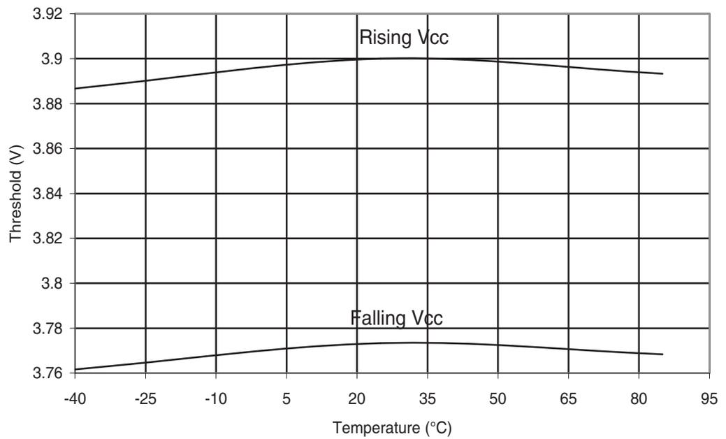
**Figure 29-37.** BOD Thresholds vs. Temperature (BODLEVEL is 2.7V)
