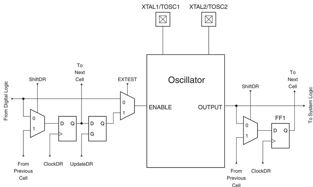
Table 25-3 summarizes the scan registers for the external clock pin XTAL1, oscillators with XTAL1/XTAL2 connections as well as 32 kHz Timer Oscillator.
