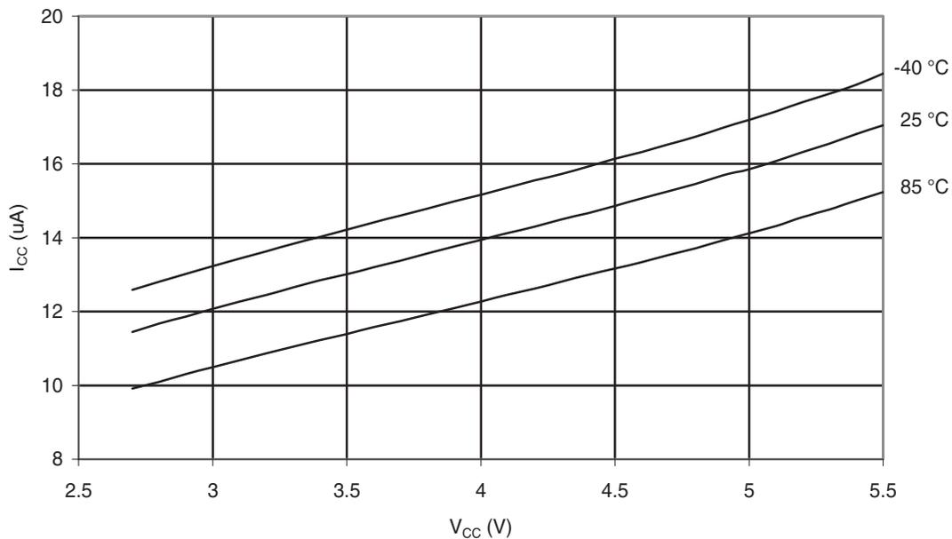
**Figure 29-53.** ADC Current vs.  $V_{CC}$  (ADC CLK = 50 kHz)
