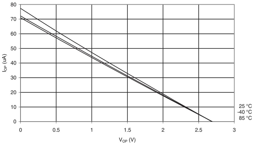
**Figure 29-22.** Reset Pull-up Resistor Current vs. Reset Pin Voltage ( $V_{CC} = 5V$ )
