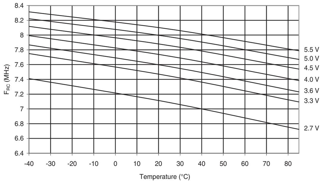
**Figure 29-50.** Calibrated 8 MHz RC Oscillator Frequency vs.  $V_{CC}$
