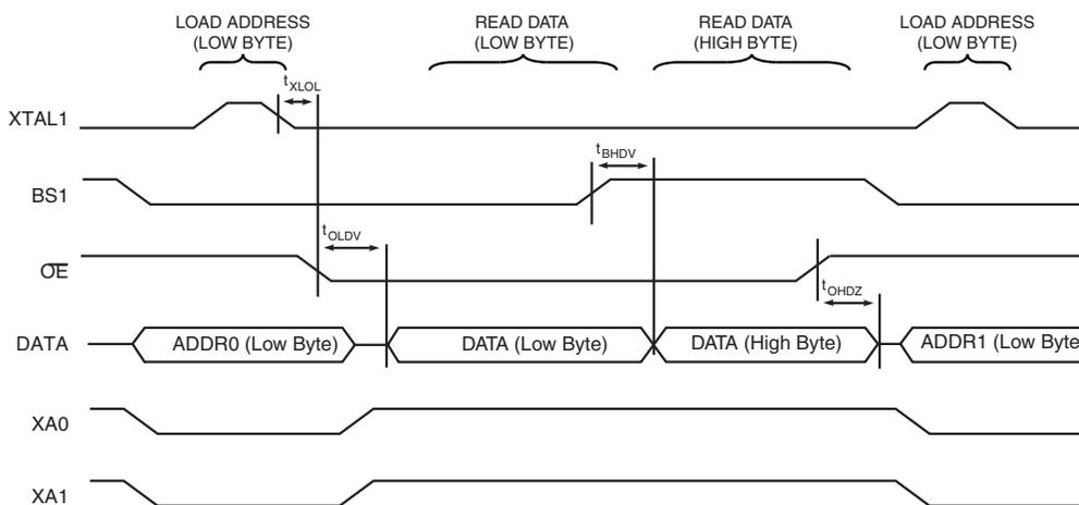
Note: 1. The timing requirements shown in Figure 27-7 (i.e.  $t_{DVXH}$ ,  $t_{XHXL}$ , and  $t_{XLDX}$ ) also apply to reading operation.
