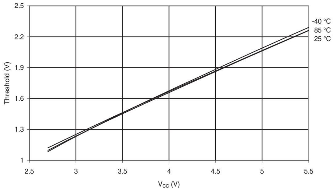
**Figure 29-32.** I/O Pin Input Hysteresis vs.  $V_{CC}$
