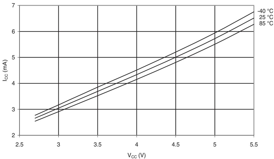
**Figure 29-6.** Active Supply Current vs.  $V_{CC}$  (Internal RC Oscillator, 8 MHz)
