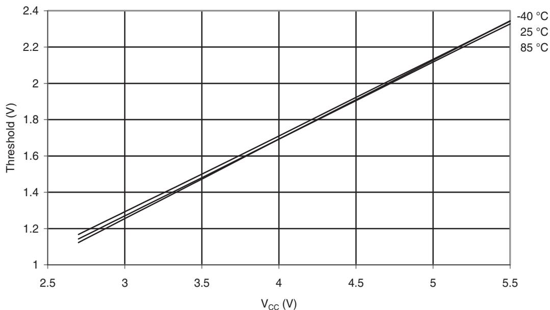
**Figure 29-35.** Reset Input Pin Hysteresis vs.  $V_{CC}$
