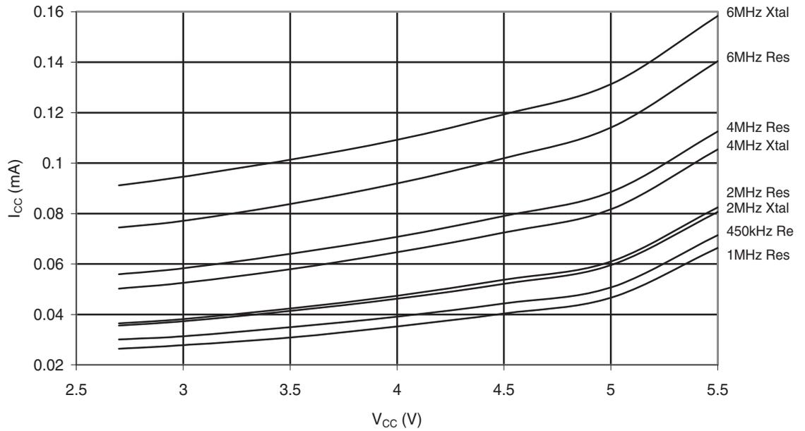
**Figure 29-19.** Standby Supply Current vs.  $V_{CC}$  (CKOPT Programmed)
