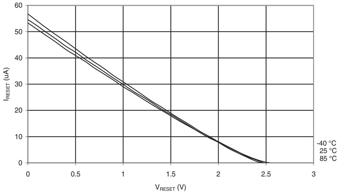
**Figure 29-24.** PEN Pull-up Resistor Current vs. PEN Pin Voltage ( $V_{CC} = 5V$ )
