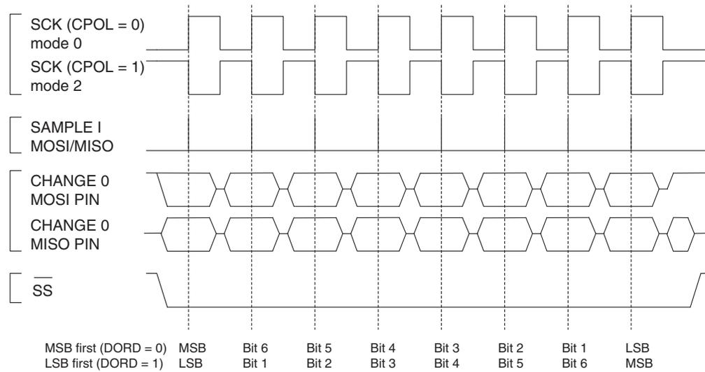
**Figure 19-4.** SPI Transfer Format with CPHA = 1
