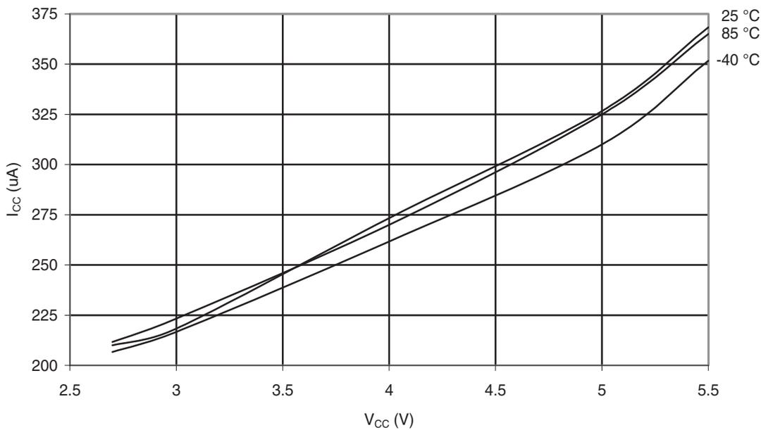
**Figure 29-54. Aref Current vs.  $V_{CC}$**
