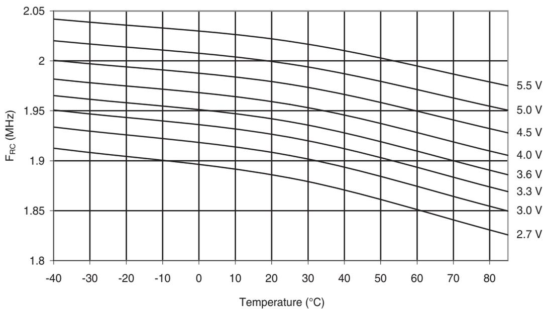
**Figure 29-44.** Calibrated 2 MHz RC Oscillator Frequency vs.  $V_{CC}$
