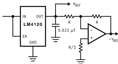
**Figure 22. Voltage Reference With Complimentary Output Circuit**
