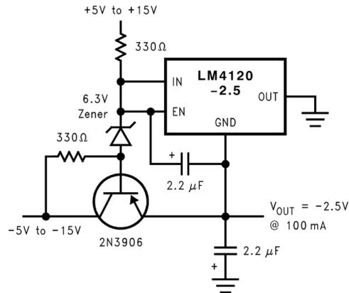
**Figure 21. Precision High-Current Negative Voltage Regulator Circuit**
