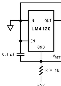
Figure 19. Voltage Reference With Negative Output Circuit
