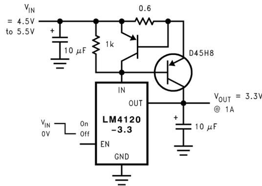
Figure 27. Precision Regulator With Current Limiting Circuit
