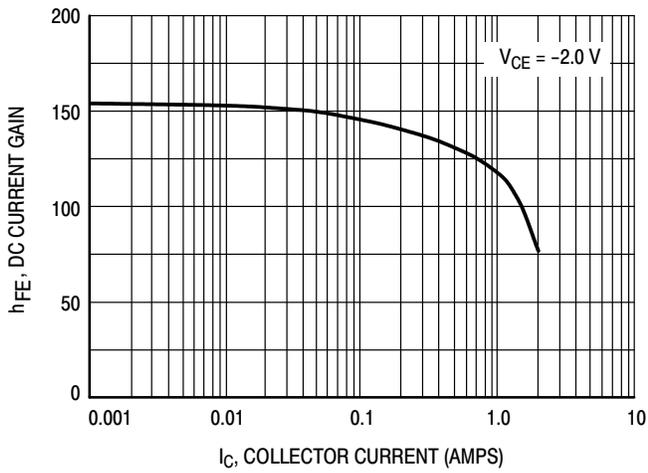
**Figure 1. DC Current Gain versus Collector Current**
