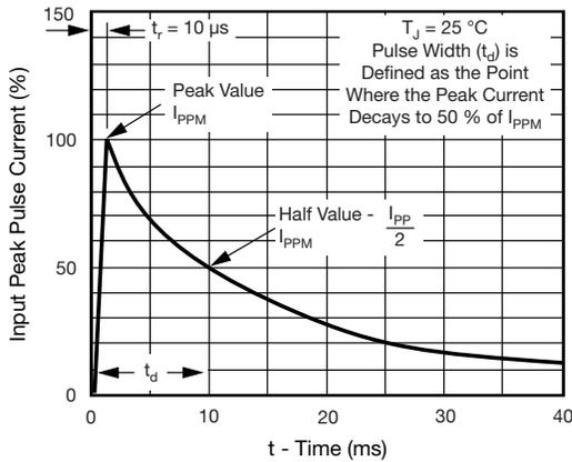
Fig. 3 - Pulse Waveform
