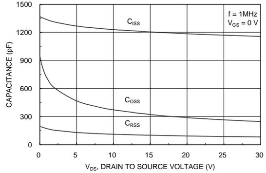
Figure 8. Capacitance Characteristics.
