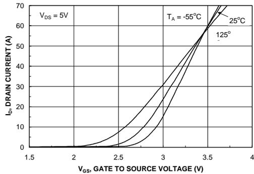
Figure 5. Transfer Characteristics.
