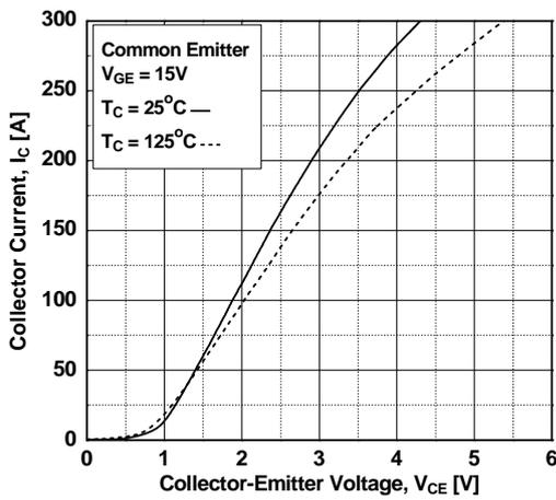
Figure 4. Transfer Characteristics
