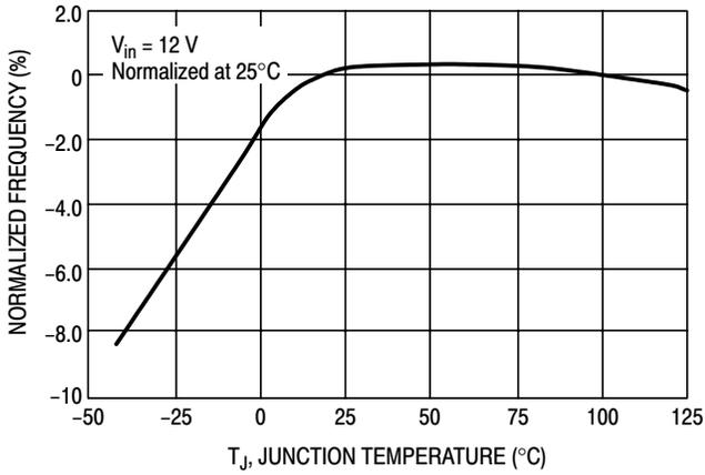
Figure 10. Oscillator Frequency
