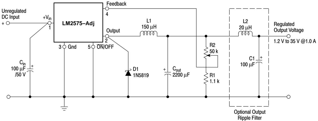
**Figure 33. Adjustable Power Supply with Low Ripple Voltage**
