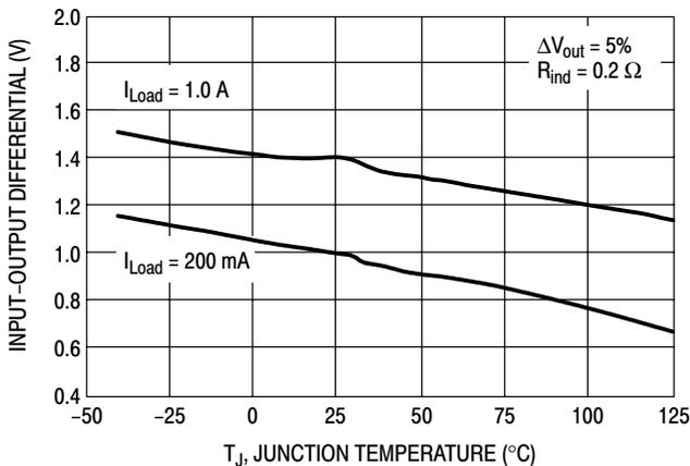
Figure 6. Dropout Voltage
