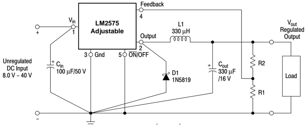
$$V_{out} = V_{ref} \left( 1 + \frac{R2}{R1} \right)$$
