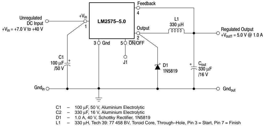
Figure 35. Schematic Diagram of the LM2575-5.0 Step-Down Converter
