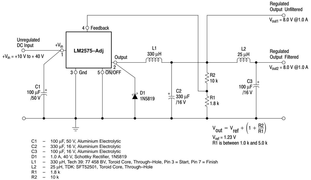
**Figure 38. Schematic Diagram of the 8.0 V @ 1.0 V Step-Down Converter Using the LM2575-Adj**
