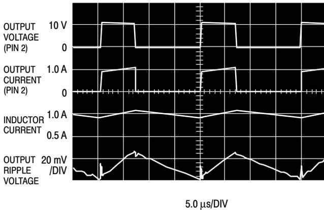
Figure 12. Switching Waveforms
