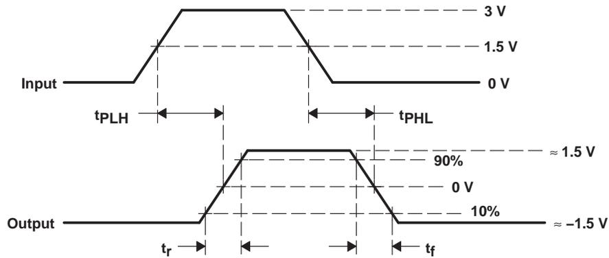
Figure 4. Output Switching Test Circuit and Waveforms
