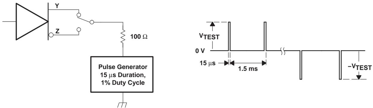
Figure 8. Test Circuit and Waveform, Transient Over-Voltage
