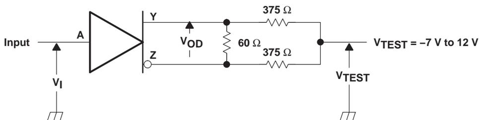
Figure 2. Test Circuit,  $V_{OD}$  With Common-Mode Loading
