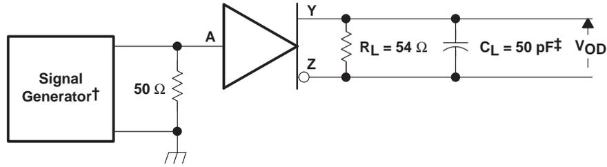
† PRR = 1 MHz, 50% duty cycle,  $t_r < 6\ \text{ns}$ ,  $t_f < 6\ \text{ns}$ ,  $Z_O = 50\ \Omega$
