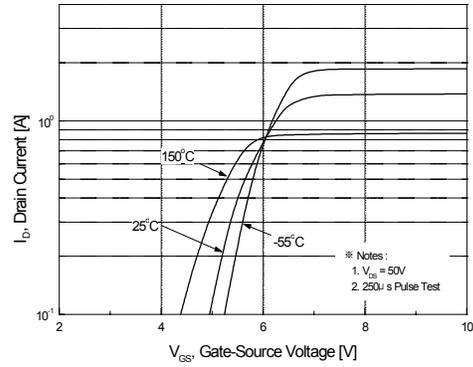
**Figure 2. Transfer Characteristics**
