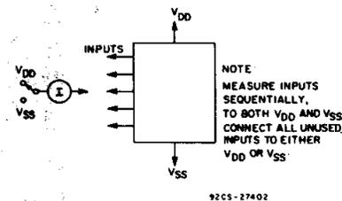
Fig. 17 — Input current test circuit.
