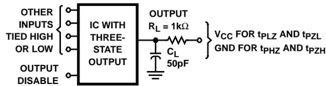
NOTE: Open drain waveforms  $t_{PLZ}$  and  $t_{PZL}$  are the same as those for three-state shown on the left. The test circuit is Output  $R_L = 1k\Omega$   $V_{CC}$ ,  $C_L = 50pF$ .
