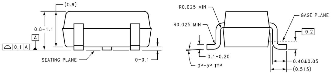
DIMENSIONS ARE IN MILLIMETERS
