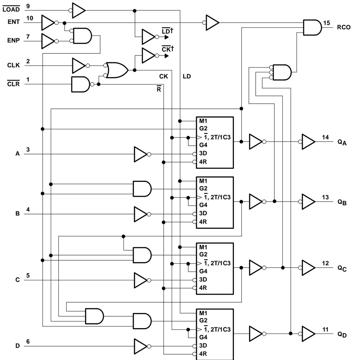
† For simplicity, routing of complementary signals  $\overline{\text{LD}}$  and  $\overline{\text{CK}}$  is not shown on this overall logic diagram. The uses of these signals are shown on the logic diagram of the D/T flip-flops.
