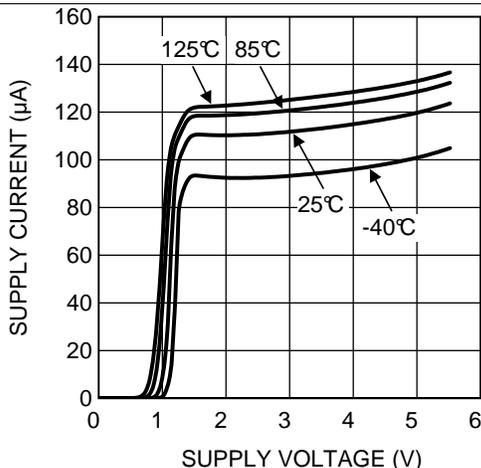
**Figure 1. Supply Current vs Supply Voltage (LMV611)**
