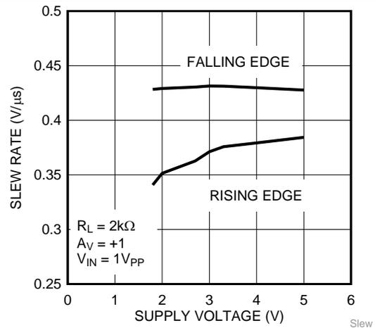
Figure 20. Slew Rate vs Supply Voltage LMV612 Only
