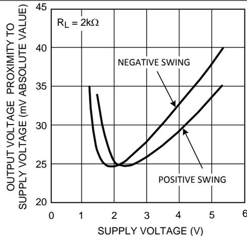
Figure 8. Output Voltage Swing vs Supply Voltage
