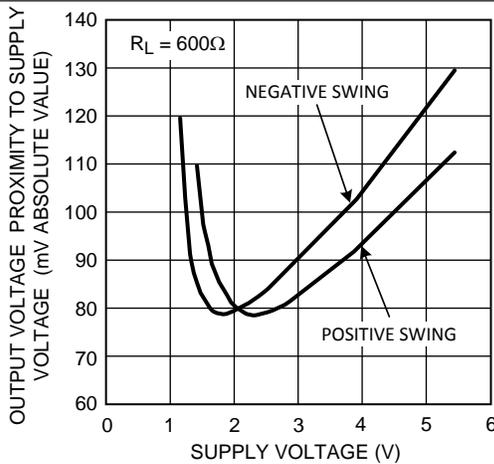
Figure 7. Output Voltage Swing vs Supply Voltage
