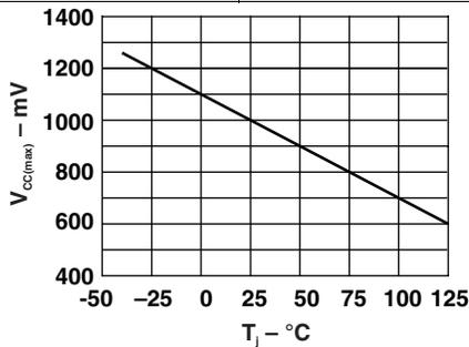
Figure 5.  $V_{CC(max)}$  vs Junction Temperature
