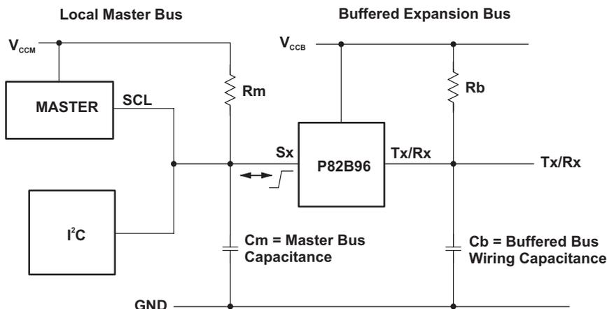
Rising edge of SCL at master is delayed (clock stretch) by buffer and bus rise times.
