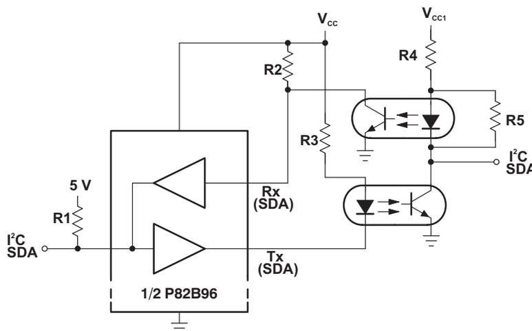
**Figure 12. Galvanic Isolation of I<sup>2</sup>C Nodes**
