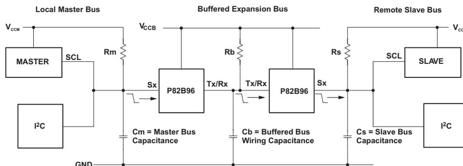
Falling edge of SCL at master is delayed by the buffers and bus fall times.
