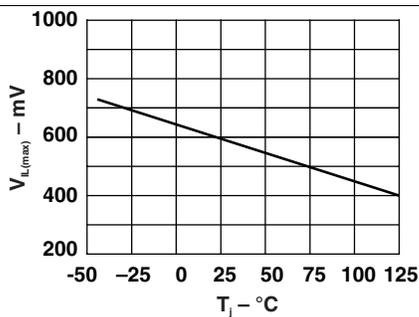
Figure 3.  $V_{IL(max)}$  at Sx vs Junction Temperature
