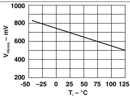
Figure 4.  $V_{IH(min)}$  at Sx vs Junction Temperature
