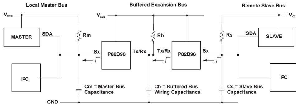
Rising edge of SDA at slave is delayed by the buffers and bus rise times.
