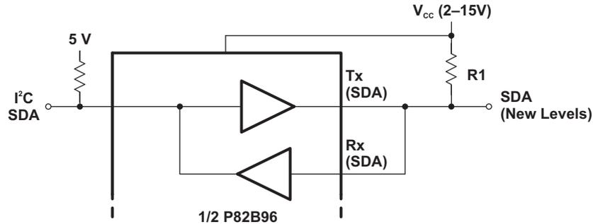
Figure 15. Interfacing I<sup>2</sup>C Bus With Different Logic Levels
