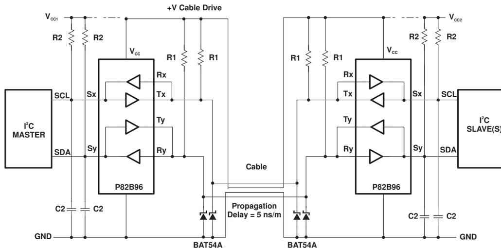
Figure 10. Driving Ribbon or Flat Telephone Cables
