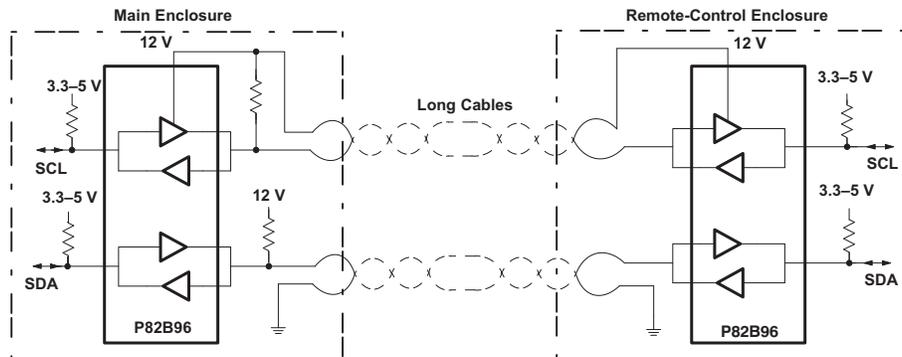
Figure 13. Long-Distance I<sup>2</sup>C Communications
