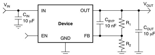
**Figure 12. Adjustable Operation for Maximum AC Performance**
