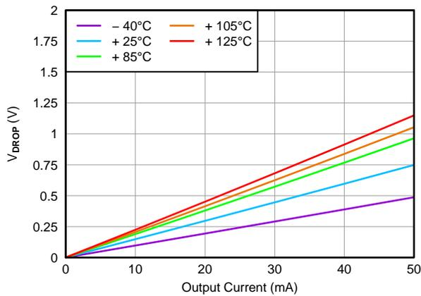
Figure 7. Dropout Voltage
