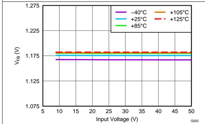
Figure 3. Feedback Voltage
