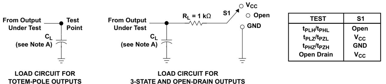
LOAD CIRCUIT FOR TOTEM-POLE OUTPUTS
