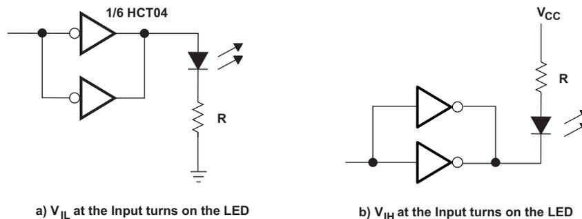
a)  $V_{IL}$  at the Input turns on the LED
