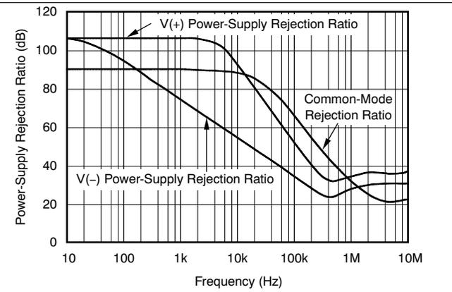
Figure 2. Power-Supply and Common-Mode Rejection Ratio vs Frequency
