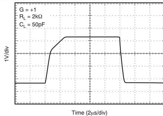
Figure 18. Large-Signal Pulse Response
