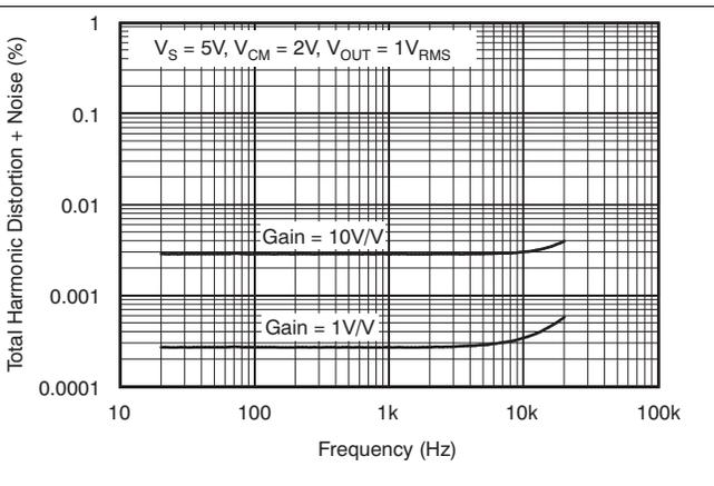
Figure 6. Total Harmonic Distortion + Noise vs Frequency
