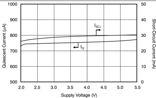
Figure 9. Quiescent and Short-Circuit Current vs Supply Voltage
