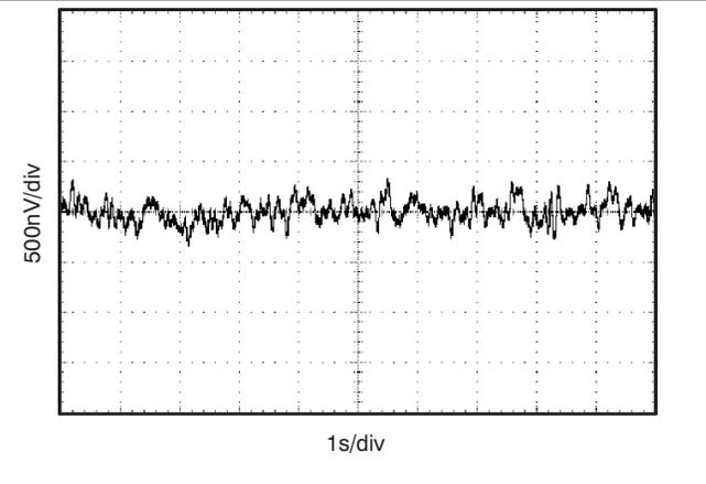
Figure 4. 0.1-Hz to 10-Hz Input Voltage Noise
