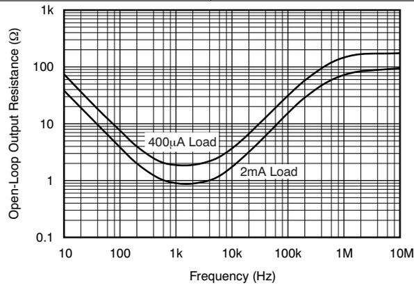
**Figure 21. Open-Loop Output Resistance vs Frequency**
