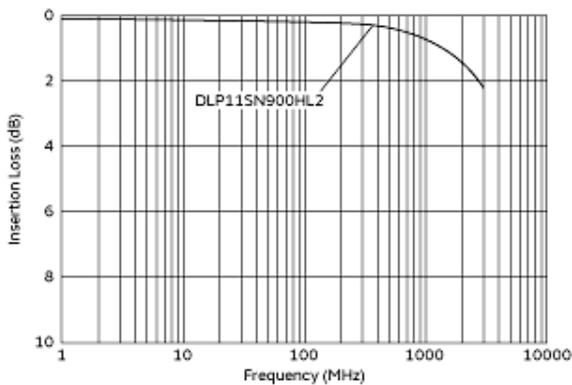
Differential Mode Transmission Characteristics (Typical Value)
